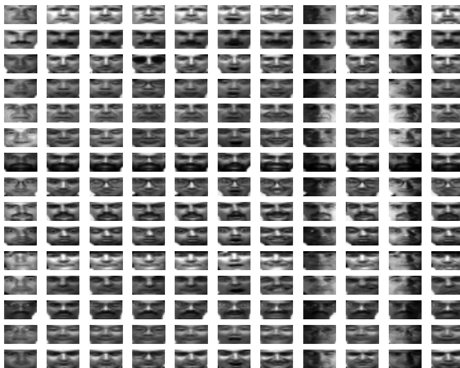
Figure 4.10 The face dataset consist of 15 subjects posing in 11 different ways, thus giving categories of: center light, no glasses, sleepy, glasses, normal, surprised, happy, right light, wink, left light and sad . Each image is 50 \times 60 pixels, thus giving a matrix \mathbf{X} size 165 \times 3000 . Eyes and mouth was center aligned by manual translocation to give the best possible overlap between faces.
