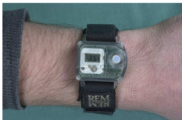
Figure 7.1 The device measuring sun radiation the skin is exposed on.
