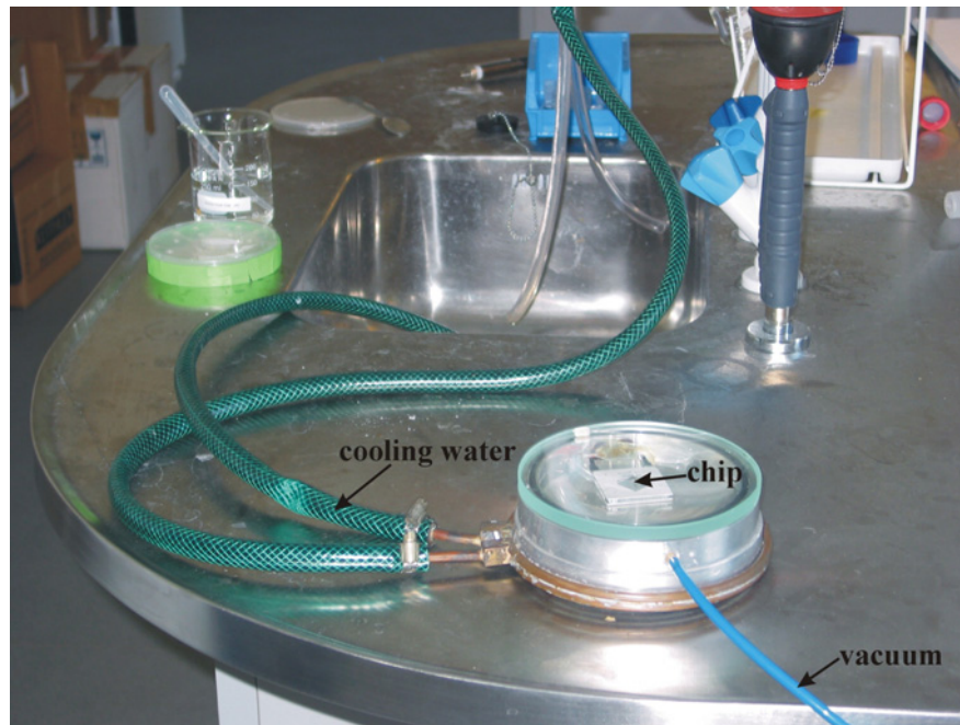
Figure 5.13: Image of the freeze drying setup where the chip is placed into a cooled vacuum chamber
