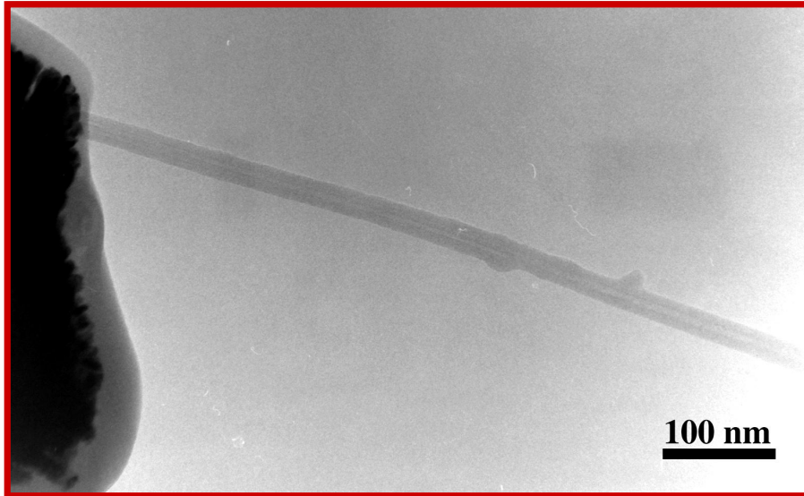
Figure 8.13: TEM image of a tip with a MWCNT assembled using the direct manipulation technique. The amorphous layer is carbon and probably deposited during the assembly. The outer diameter is approximately 24 nm and the inner tube(s) is 6-7 nm wide. Image by Frans D. Tichelaar, TUDelft
