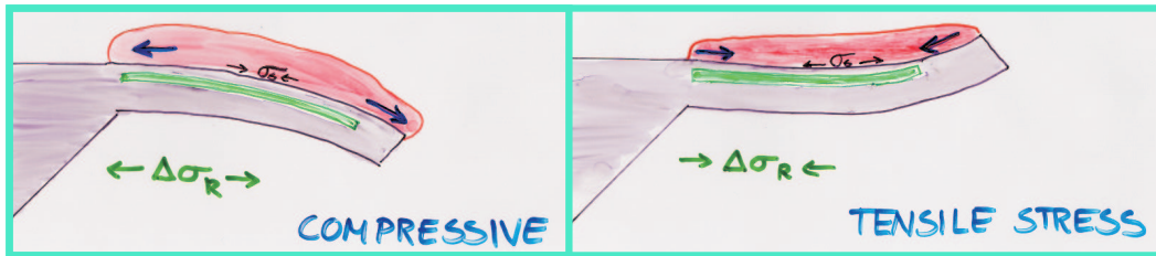
Figure 2.6: Stress in a film on a cantilever. As the film expands the cantilever is bent down giving rise to a tensile stress in the resistor. The resulting stress in the film is compressive as its expansion is hindered and balanced by the bending of the beam. Conversely, for a contracting film the cantilever bends up and the resulting stress in the film is tensile.
