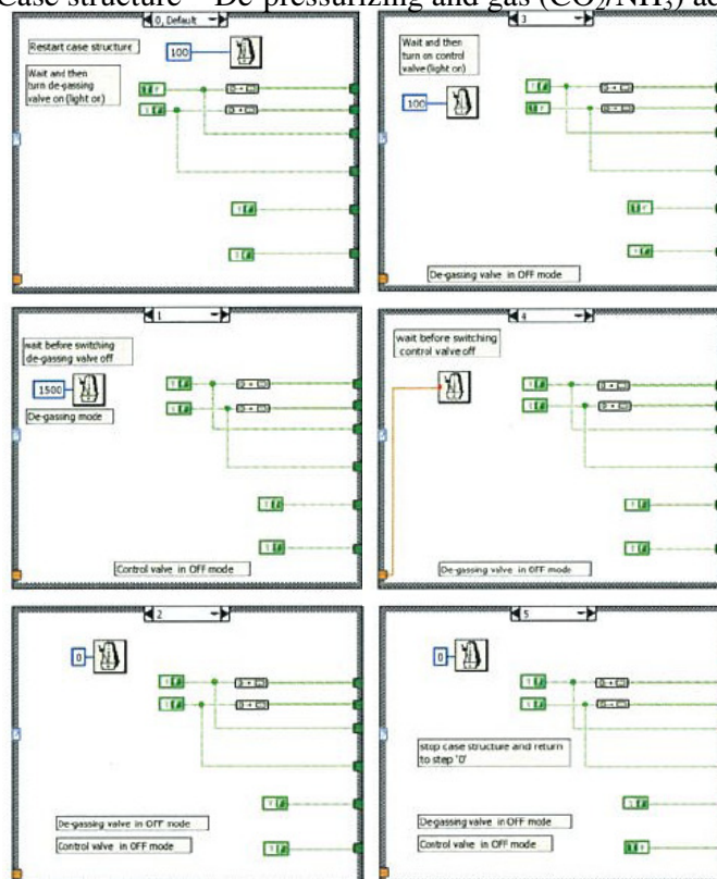
Case structure – De-pressurizing and gas ( CO_2/NH_3 ) addition sequence.
