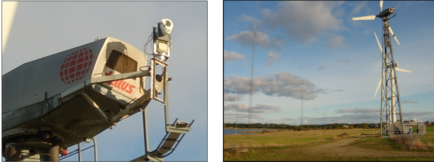
Figure 9. The wake measurement experimental set-up at Risø Test Center at Roskilde Denmark. Left: The prototype lidar mounted at the back of the Tellus turbine. Right: The field view. The 30 m tall meteorological mast is located in the dominant wind direction 37 m away from the turbine.
