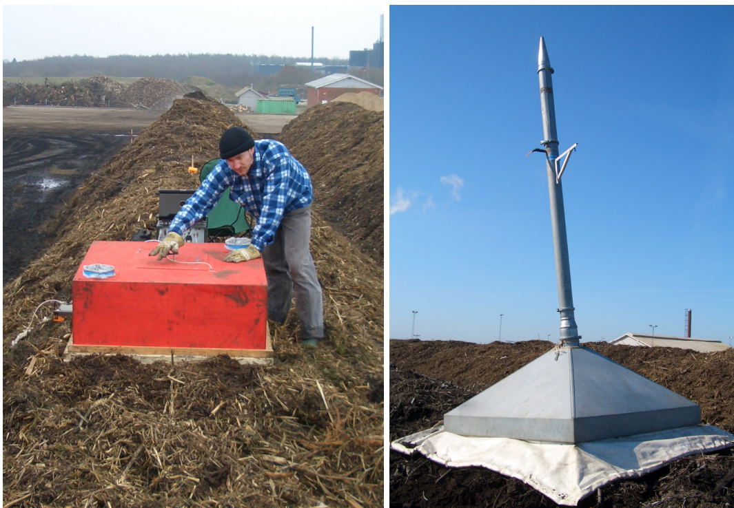
Figure 5. Pictures of the two small-scale measurement methods used at the composting plant in Aarhus, Denmark, namely the static flux chamber (left) and the funnel method (right).
