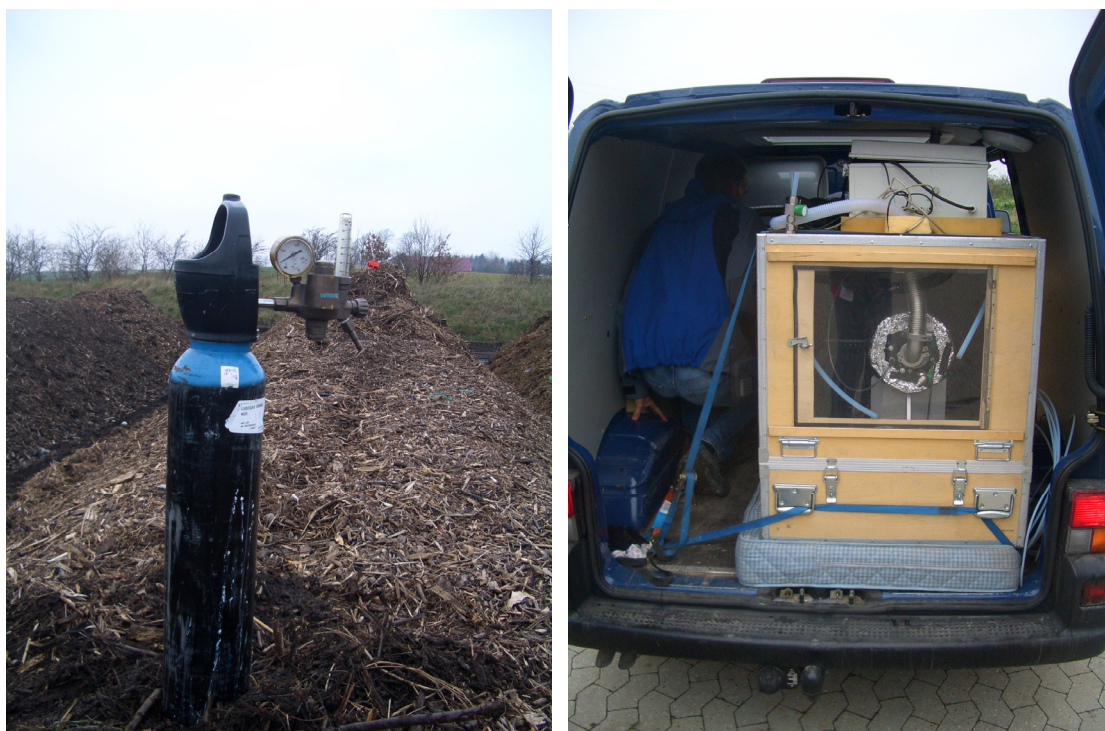
Figure 6. Pictures of the dynamic plume method. Left: Tracer gas release on top of the windrow. Right: Fourier Transform Infra-Red (FTIR) measurement system incorporated in a van.
