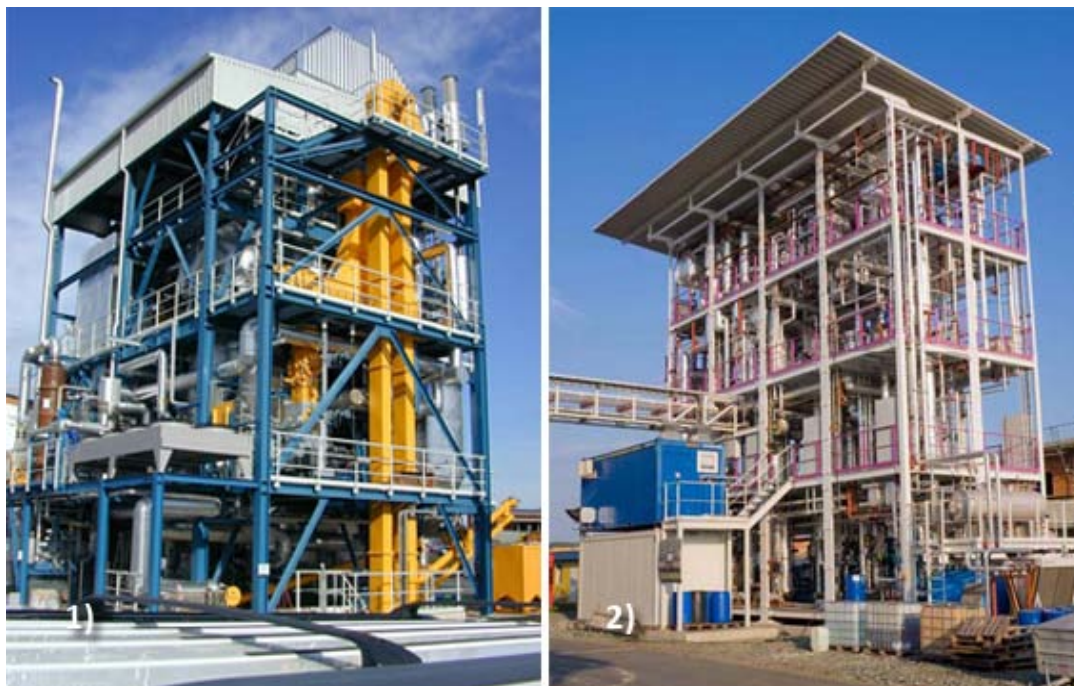
Figure 3-9: Picture 1) 8 MW biomass FICFB gasifier for heat and power production. Picture 2) 1 MW SNG FICFB PUD for SNG production from biomass (PSI, 2009)
