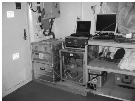
Figure 2. The LC&R S-38 marine gravity meter in “the hangar”. The LC&R land gravity meter G-867, which was used for the harbour ties, is stored in an aluminium box and strapped to the lower shelf next to the marine meter.
