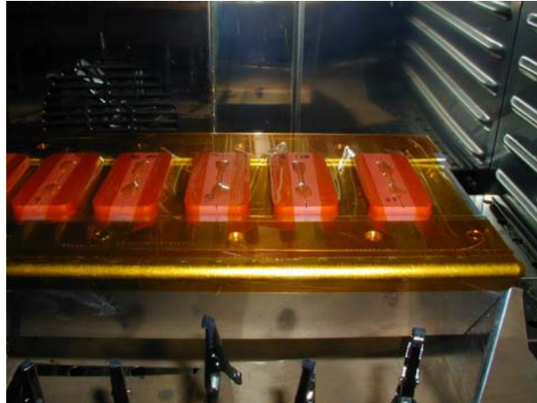
Figure 4: Pre-straining set-up. The weights are fixed onto the fiber with metallic clamps.
