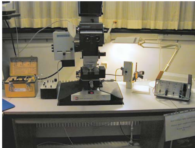
Figure 7: Test set-up. From left side: Strain measurement box, which is connected to one of the specimen holders, switch box with push and pull switch and speed regulator connected to the motor, microscope with test apparatus, motor connected with a wire to the tensile tester, electrical current box.
