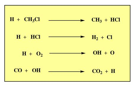
In the case that the producer gas is to be used on gas engines the intermediacy of chlorine atoms in the combustion process may lead to accumulation of covalently bound chlorine in the lubricating oil.
