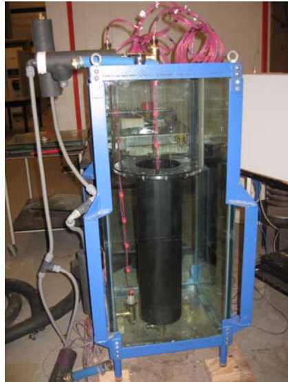
Fig. 3-2. Picture of the tank-in-tank heat store. The inner tank is for domestic hot water, whereas the outer tank is for water for space heating.
