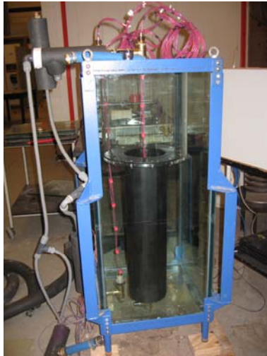
Fig. 2-46. Tank-in-tank heat store photo and inner dimensions.
