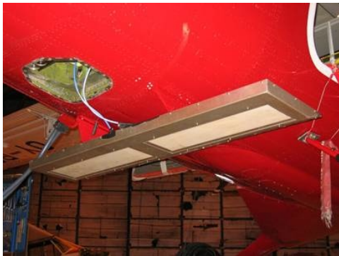
(b) ASIRAS antenna mounted in front of the opening for the laser scanner.
