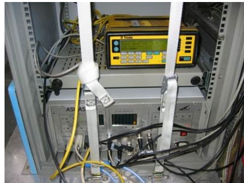
(c) ASIRAS instrument installed in the rack with a GPS instrument (Trimble 4000).
