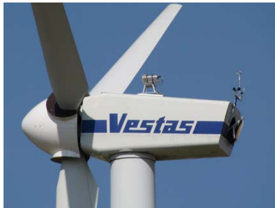
Figure 2: ZephIR lidar's optical head mounted on the V27 wind turbine's nacelle
