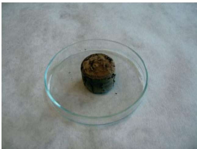
Figure 1. Photographic image of the brown solid obtained after hydrothermal treatment of a mixture of sucrose and ammonia in a Teflon beaker. The porous carbon maintains the shape of the beaker.
