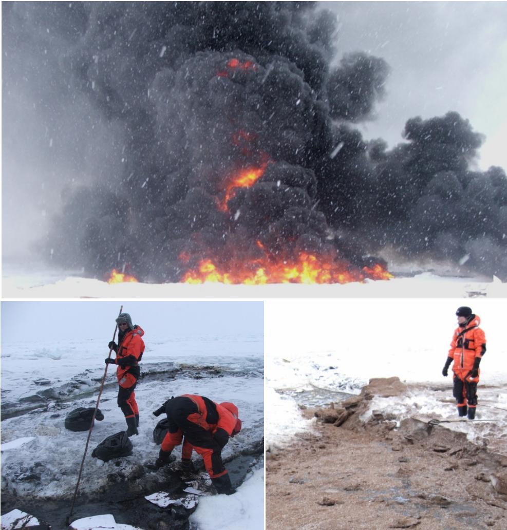
Figure 4.4.1 Large-scale in situ burning in the Barents Sea (top), collecting of residue with 3M absorption pads (lower left) and sphagnum peat moss applied to the area after the residue has been removed (lower right, photo: Per Johan Brandvik).
