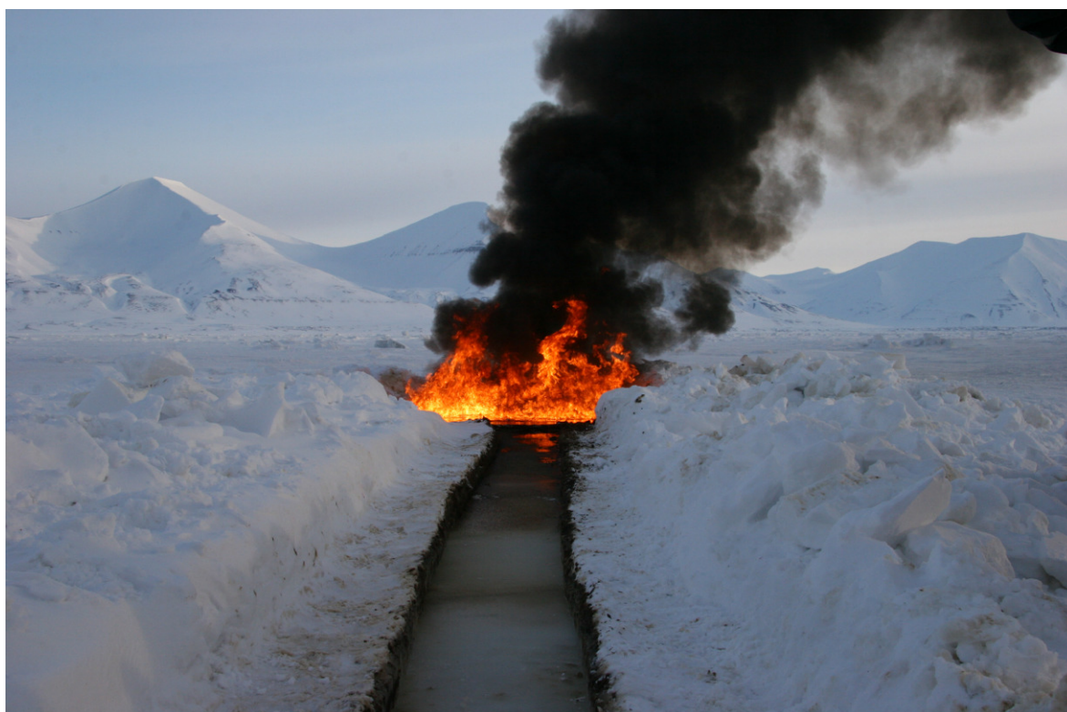
Figure 4 ISB of weathered oil.
