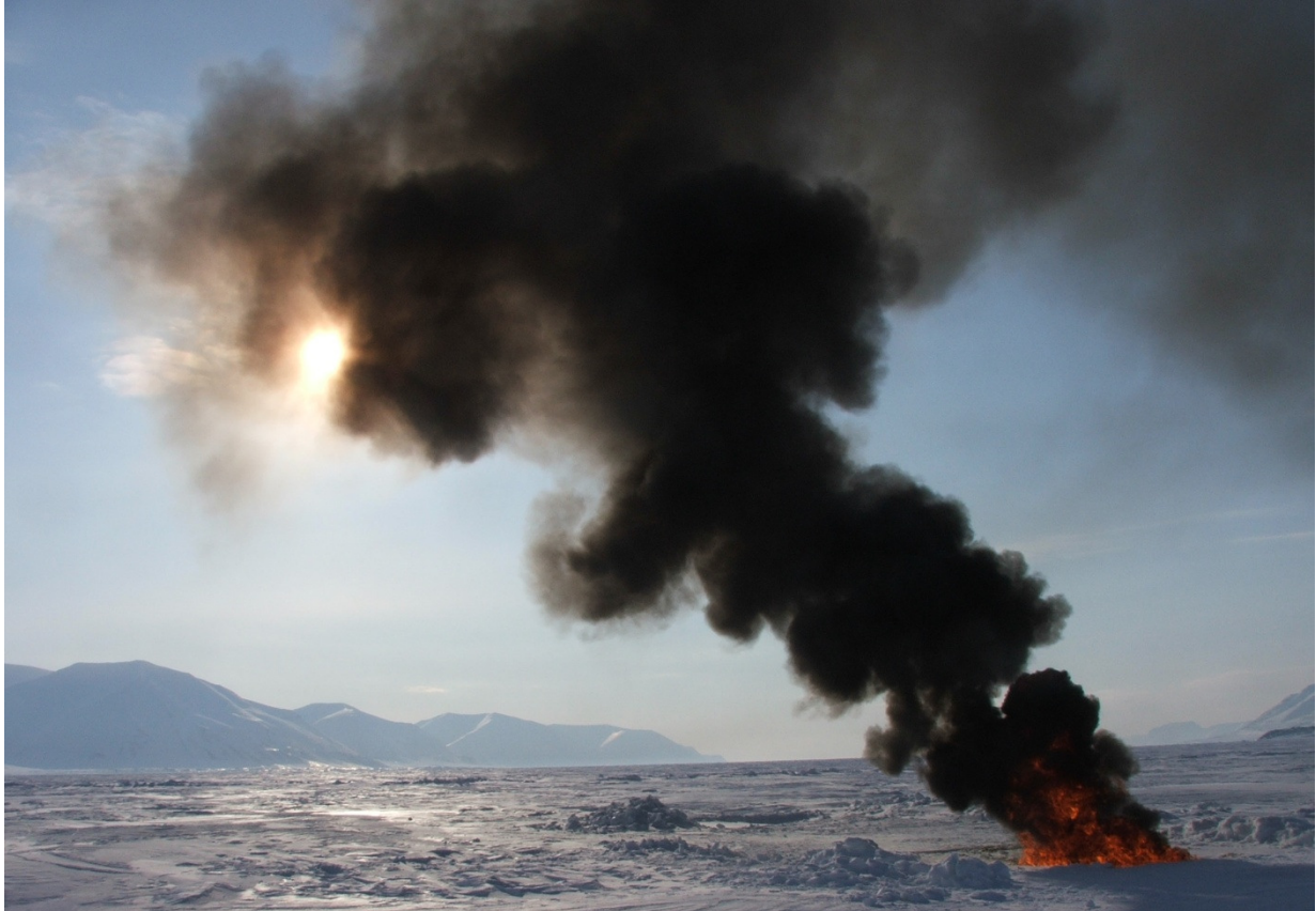
Figure 2.6.1 Smoke plume from burning Troll B crude oil in a basin cut in the fjord ice, Svea, Svalbard, 2008.
