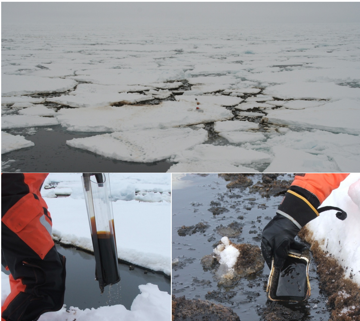
Figure 3.2.5 Weathering experiment with Troll B crude oil in the marginal ice zone in the Barents Sea at the beginning of the experiment (top). Measuring the oil slick thickness (bottom left) and sampling (bottom right).
