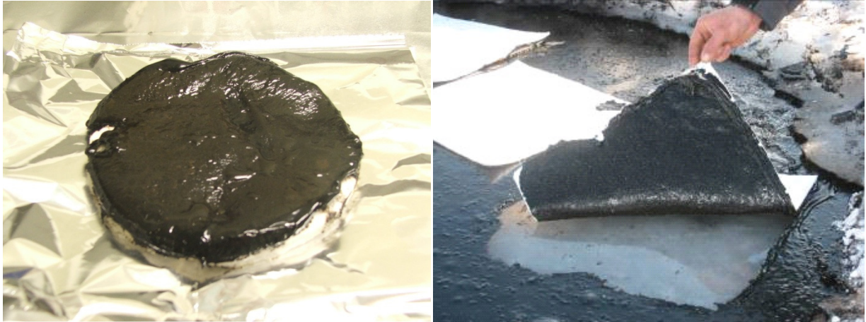
Figure 2.5.1 Examples of burn residues from the laboratory (IFO-30) and the field (Statfjord) (right photo: Per Johan Brandvik).
