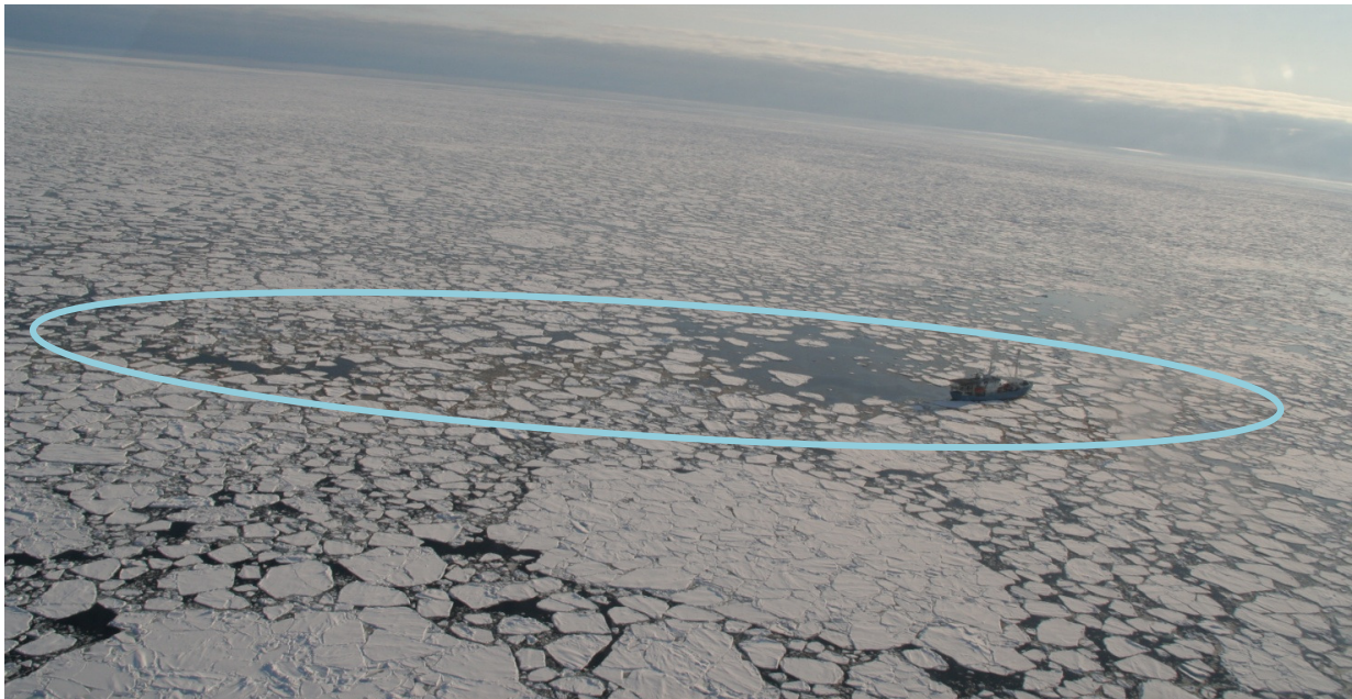
Figure 4.3.3 The 7000 L oil spill in the ice in the Barents Sea at the end of the experiment six days after the release. The slick had spread out and covered an area of 100 m x 3000 m. The research vessel Lance is seen to the right in the picture.
