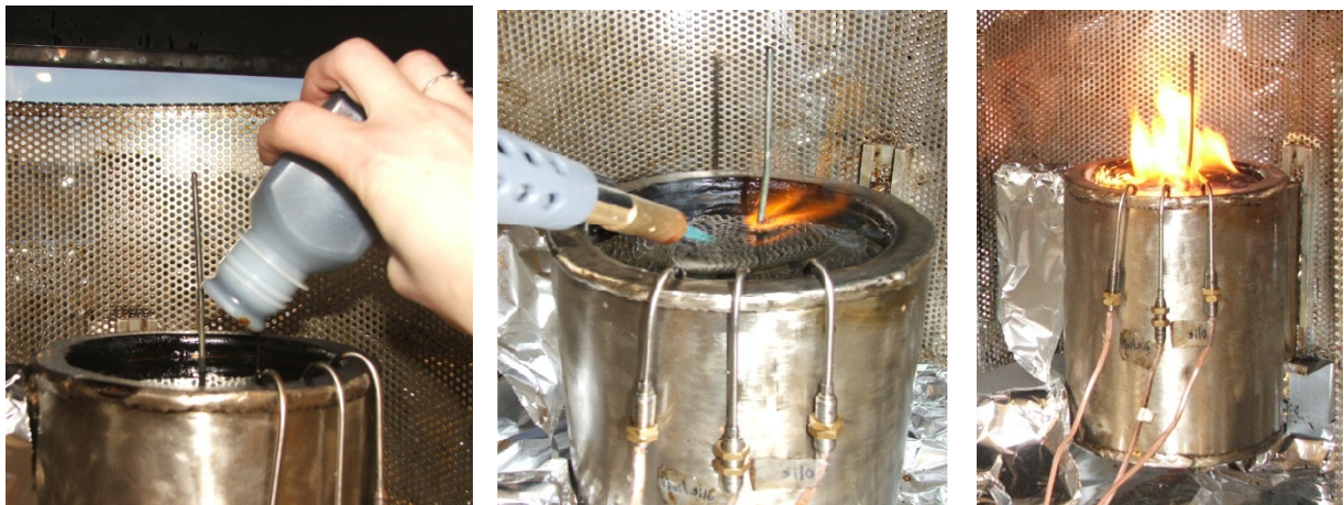
Figure 3.3.1 Applying (photo: Per Johan Brandvik), ignition (photo: Per Johan Brandvik) and burning of an oil sample in the laboratory burning cell.
