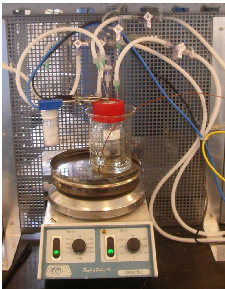
Figure 6.5: Photograph of one particular ‘incarnation’ of the old setup. The cell (inner glass vial), in this case is entirely contained inside the outer glass vial (i.e., it contains both a cathode and an anode unlike the configuration shown in Fig. 6.4). This vial sits inside a larger glass (with the red GL45 cap), which is continually purged with argon. The purpose of this outer container is to minimize the leakage of air through any possible leak in the septum of the inner cell. The outer glass container stands in an open beaker with some silicone oil to help transfer heat from the hotplate below. A thermocouple is used to measure the temperature of the silicone oil.
