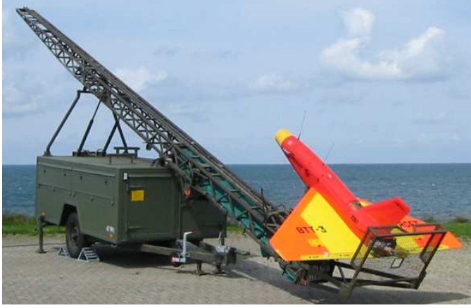
Fig. 1. Banshee UAV ready for launch at the Danish Naval Weapons School at Sjællands Odde. (Foto: VFD)
