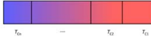
Figure 5.1: A schematic of the grading of an AMR. The color map shows the cold end (blue) and the hot end (red) as well as n different materials comprising the regenerator.
