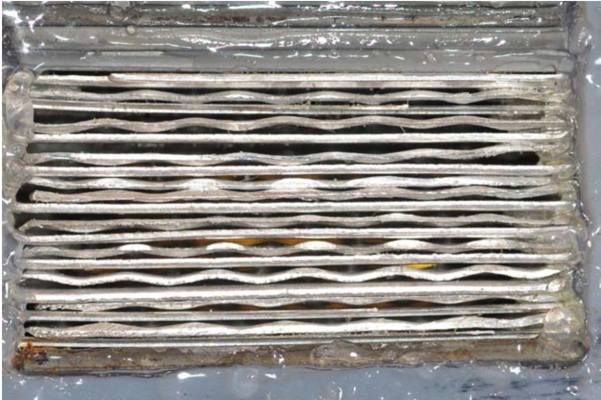
Figure 1. The dimpled plate regenerator assembled in the regenerator housing
