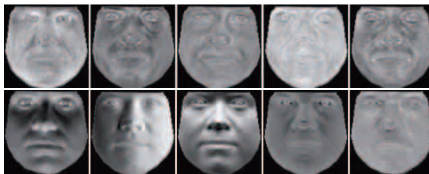
Figure 5. The first five PCA basis images of the identity and illumination subspaces. Upper row is the identity, and the lower row shows the illumination eigenfaces.
