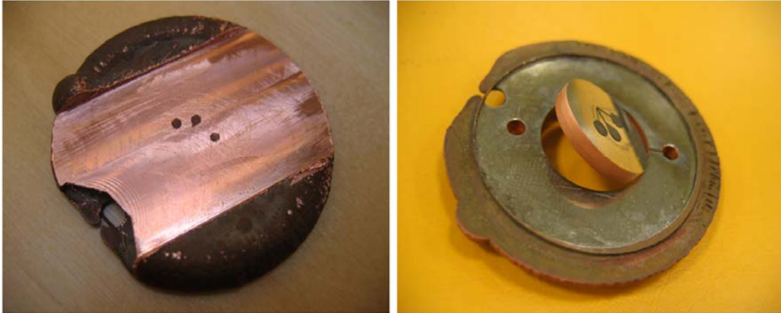
Figure 84 – Milling of the back side of the tool (left) and wire-EDM cut for final shape definition (right). The double layer composed by Cu and Ni is visible from the side of the micro tool.
