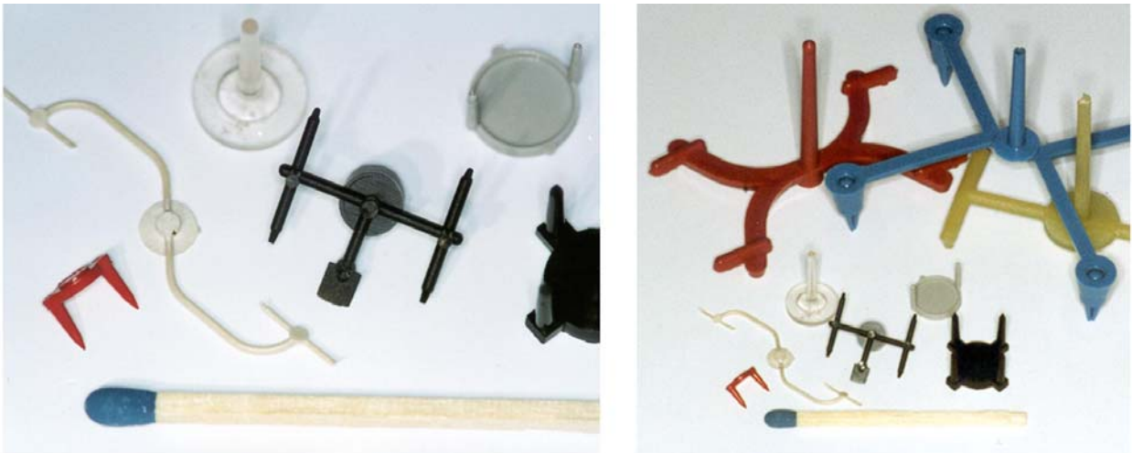
Figure 4 – Comparison of runner systems to mould micro part with conventional injection moulding machines (right) and with micro injection moulding machine (left) [Ganz, 2005].
