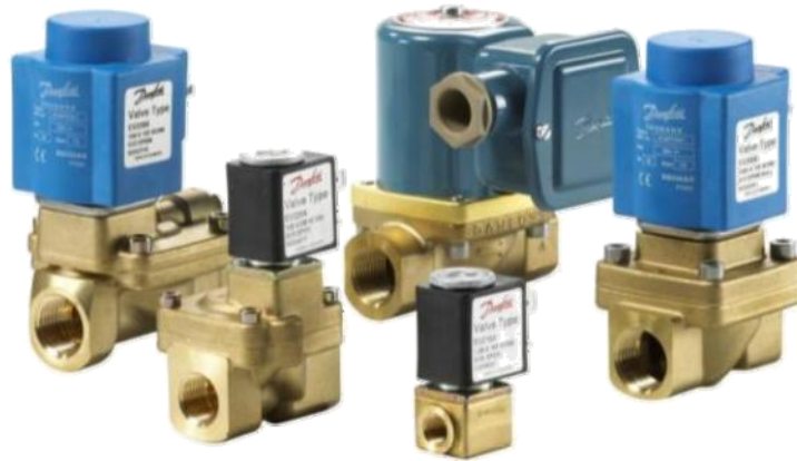
Figure 5.27: Typical automatic industrial controls valves. Note the thread connections. They are the typical way to mount industrial valves to the pipeline. The valves on the picture are used for water, oil, steam and other pipelines. The blue and black parts are the coils.
