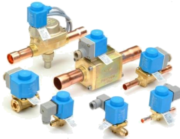
Figure 5.25: A typical series of different refrigeration solenoid valves. Note the copper tubes. They are typical refrigeration connections, soldered to the pipeline in a refrigeration system.
