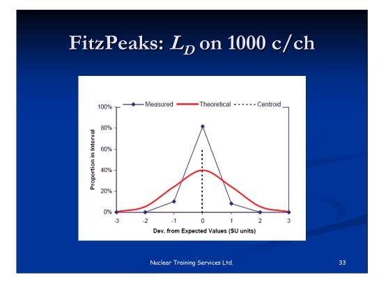
This is the distribution of area differences (measured-actual) for a FitzPeaks analysis of the Limit of Detection peaks on a 1k counts/channel background.
