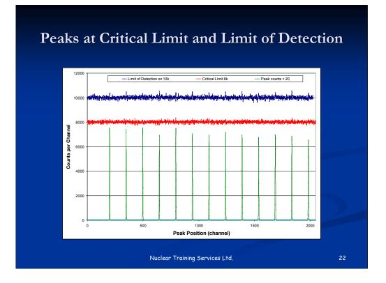
At the top is part of a spectrum containing 50 peaks on a 10k background that contain exactly the number of counts equivalent to the 95% confidence Limit of Detection.
