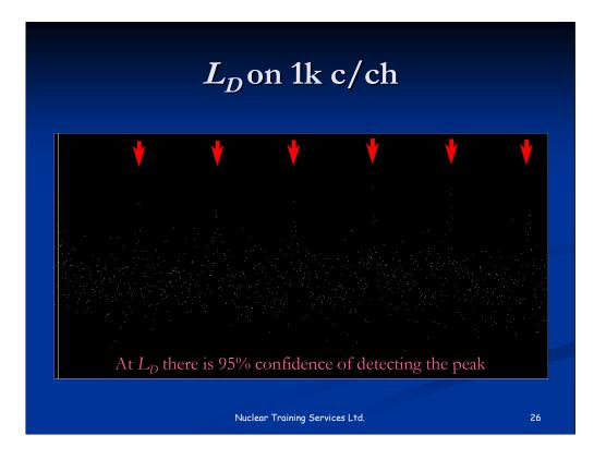
This shows part of the upper spectrum I showed you before – each peak has the number of counts corresponding to the limit of detection on a 1000 ct/channel background.
