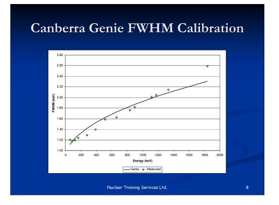
In fact, of course, this is a peak width calibration – in fact it is part of the data within the calibration spectrum provided as an example with the Genie-2000 software.
