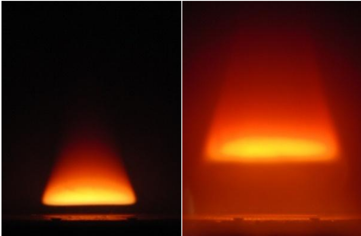
Figure 14. Pictures of stable, lifted flames. Left: Approx. 7 mm flame lift at the condition \text{CH}_4 = 8 SLM, \text{O}_2 = 5 SLM, \phi = 3.2 and camera shutter speed = 1/640 s. Right: Approx. 34 mm flame lift at the flame condition \text{C}_2\text{H}_4 = 6.3 SLM, air = 30 SLM, \phi = 3 and camera shutter speed = 1/20 s.
