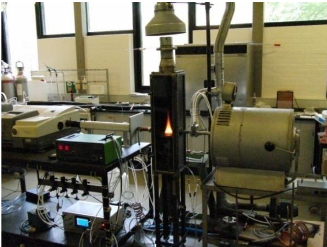
Figure 5. View of the experimental setup. The flame chamber is aligned with a Nicolet 6700 FT-IR (left) and a black body (right) to investigate radiation and absorption of the flame. A Hovagas G6 gas mixer (bottom) is used control the gas flows to the burner.
