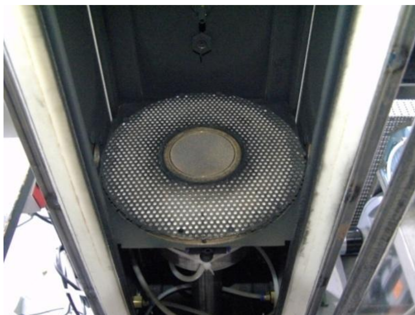
Figure 4. Top view of the standard bronze Holthuis & Associates burner surrounded by a homemade co flow screen.
