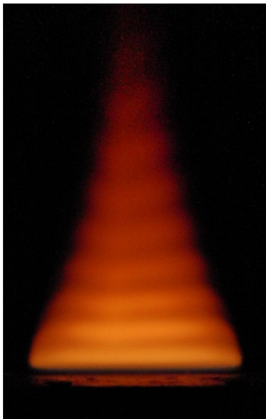
Figure 9. Image of rotating flame instability at O_2 = 6 SLM, CH_4 = 8 SLM, \phi = 2.33 and camera shutter speed = 1/640 s.
