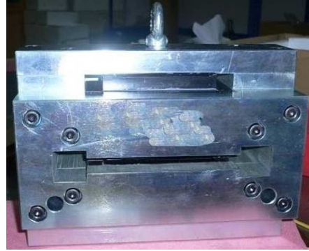
Fig. 4.10: The magnet design by Tagliafico et al. (2009). The magnetocaloric material passes through the gap in the structure.
