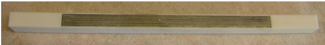
Figure 6: One of the 24 compartments from the regenerator. The one shown contains a stack of Al plates.
