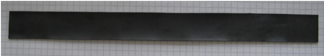
Figure 2: Graded Plate of LCSM 250 mm x 20 mm x 0.3 mm. The plate is cut from a larger sheet, tape cast in one piece, consisting of 10 discrete regions of LCSM.
