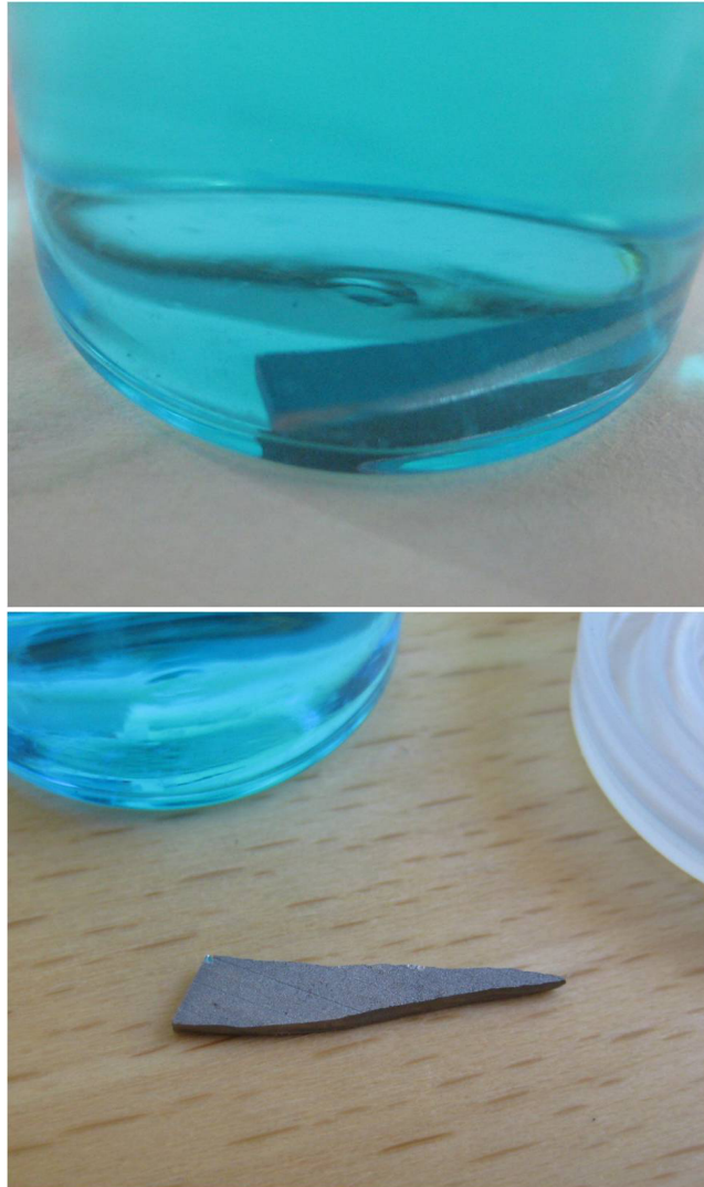
Figure 5.3: Top: Sealed container with LFCS sample and a 25% antifreeze/75% water mixture. Bottom: Untarnished sample after almost two years.
