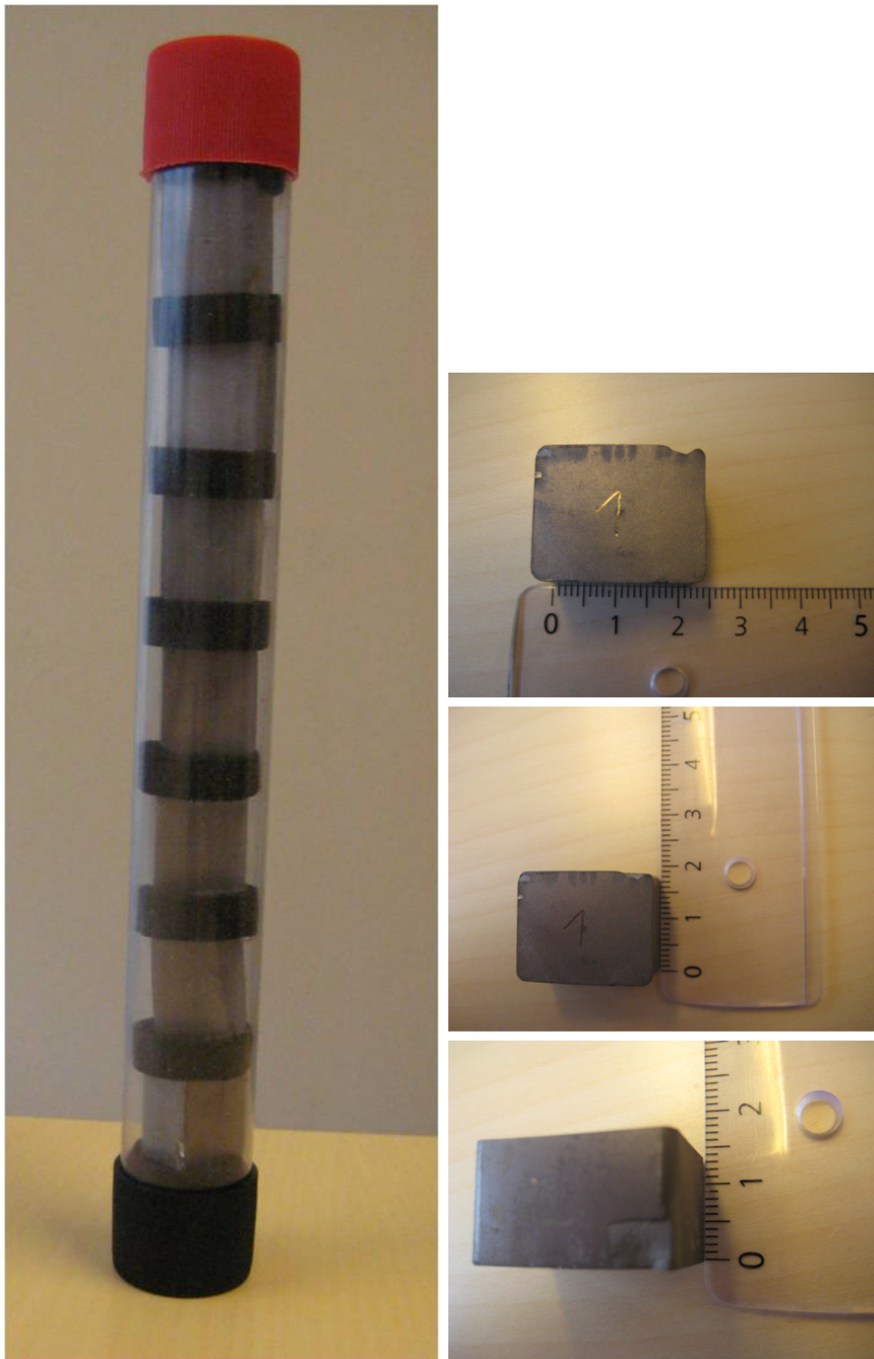
Figure 5.2: Blocks measuring approximately 23 mm \times 19 mm \times 12.5 mm produced by Vacuumschmelze GmbH. The blocks were cut into smaller pieces for experimental work, as discussed in section 5.2. The characterization of these seven samples is the subject of paper II.
