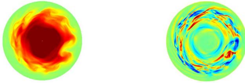
Figure 2. Snapshot of the 2D density (left) and vorticity (right) variation taken from DIESEL. Plasma parameters similar to TCV parameters.
