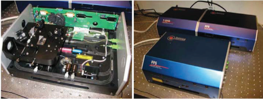
Figure 5.5: Dual-laser FFS femtosecond laser system from Toptica. Left image shows an inside view of one of the two lasers. Right image shows the two lasers on an optical table. The laser in front will drive the 32 THz detectors and the laser in the back will drive the 32 THz emitters.
