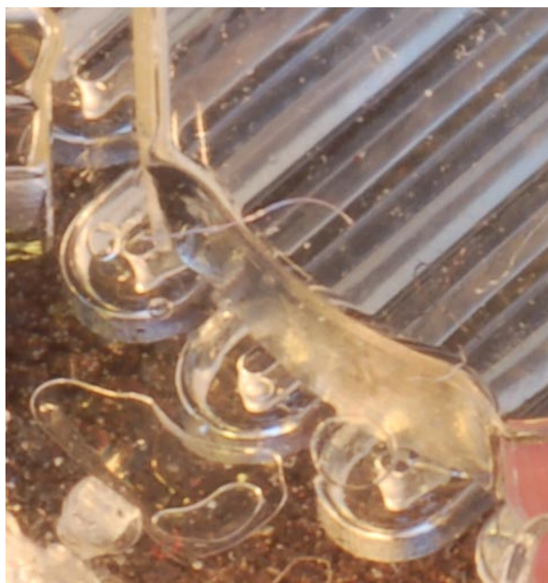
Figure 3.5: The meandering aeration channel (located in the aeration layer, here on the bottom) is only separated from the reactor chamber (side wall visible in the middle of the picture) by a membrane (not visible).
