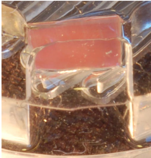
Figure 3.6: The carrier layer of the DO sensor spot (red) is attached to the inside wall of the reactor chamber whilst the active (fluorescent, black colour) layer is in direct contact with the broth. The measurement is done through the reactor wall (window thickness 1 mm).
