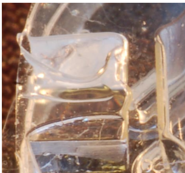
Figure 3.7: The carrier layer of the pH sensor spot (white) is attached to the inside wall of the reactor chamber whilst the active (fluorescent, yellowish colour) layer is in direct contact with the broth. The measurement is done through the reactor wall (window thickness 1 mm, located in the right half of the picture).
