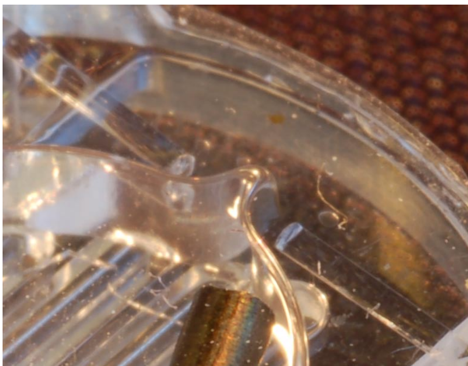
Figure 3.11: The tunnels made during fabrication are now filled with the optical fibers. The tunnel ends short of the reactor chamber creating a window through which the light reaches the chamber. The chamber has a protrusion to allow for a defined measurement path length.
