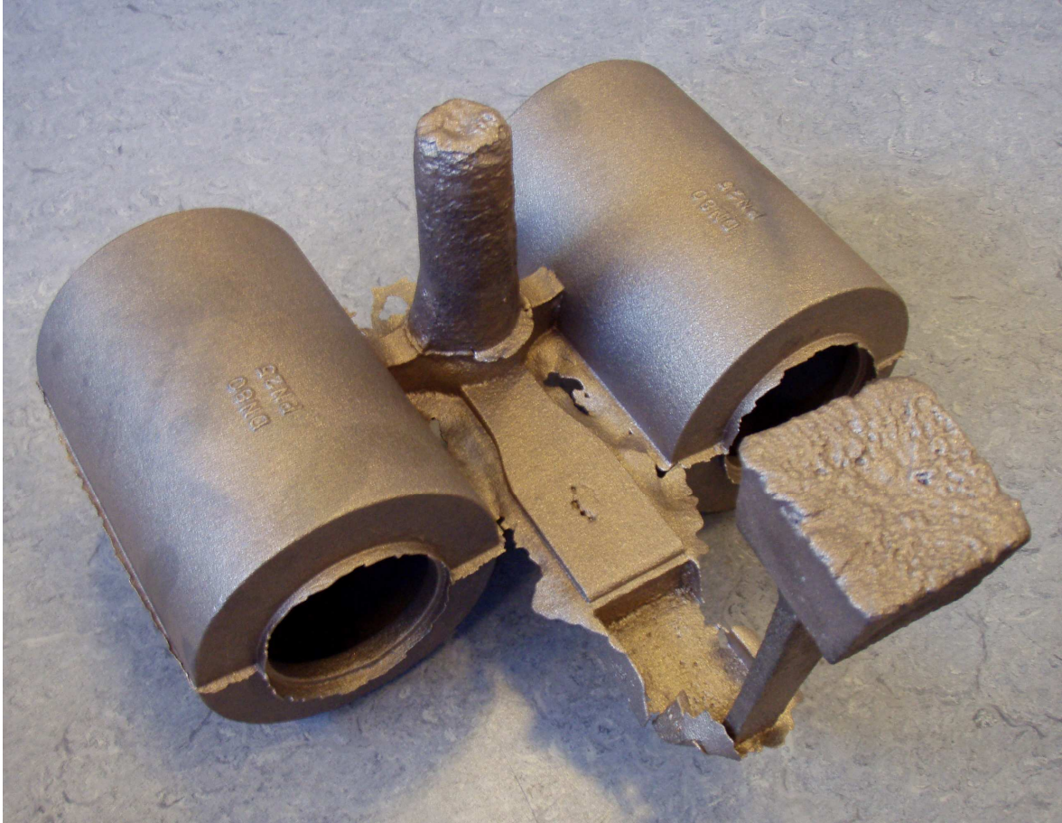
Figure 10-7 An example from one of the fully cast moulds.
