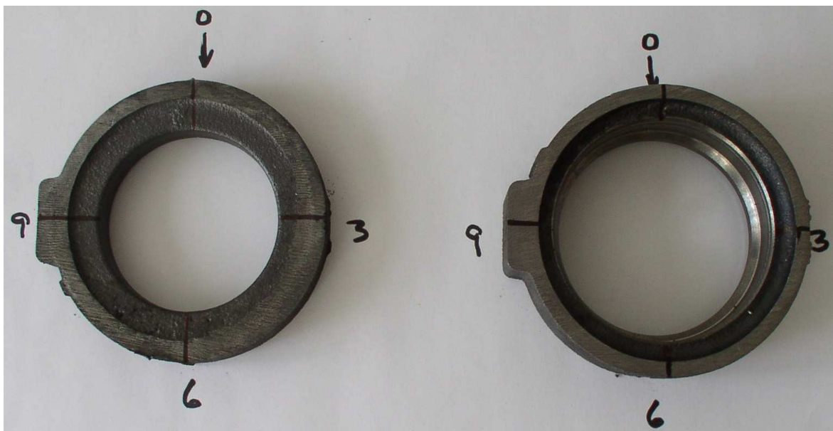
Figure 6-4 The picture shows the two centre flanges and the numbers indicates the numbering and the positions of the samples. To the left: Centre flange from the streamlined layout. To the right: Centre flange from the traditional layout.
