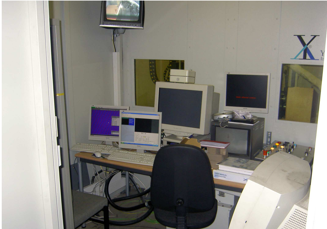
Figure 5-8 Control room with all the different computers for monitoring, filming, and recording of data.
