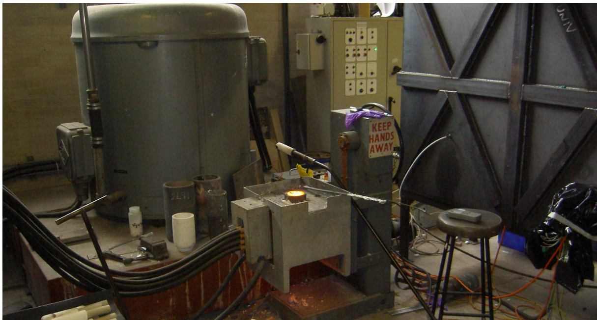
Figure 5-5 The furnace for melting
