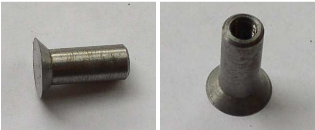
Figure 5-3 Guide pin designed for mounting the individual modules on to the base pattern plate. The length of the pin is 15mm.
