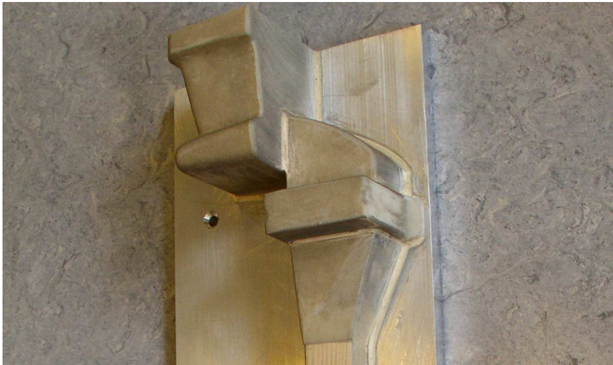
Figure 8-7 The picture shows an example of how the filter prints have been slightly modified to do the glass plate experiments. In the original use of the filter print shown here the parting line would have been perpendicular to how it is used here.
