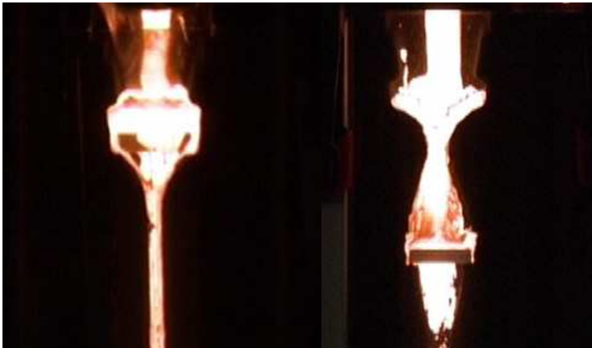
Figure 8-9 The two frames show how the melt is divided into smaller streams when using pressed filters.
