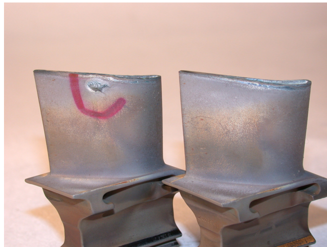
Fig. 2: Turbine blades with surface defect.
