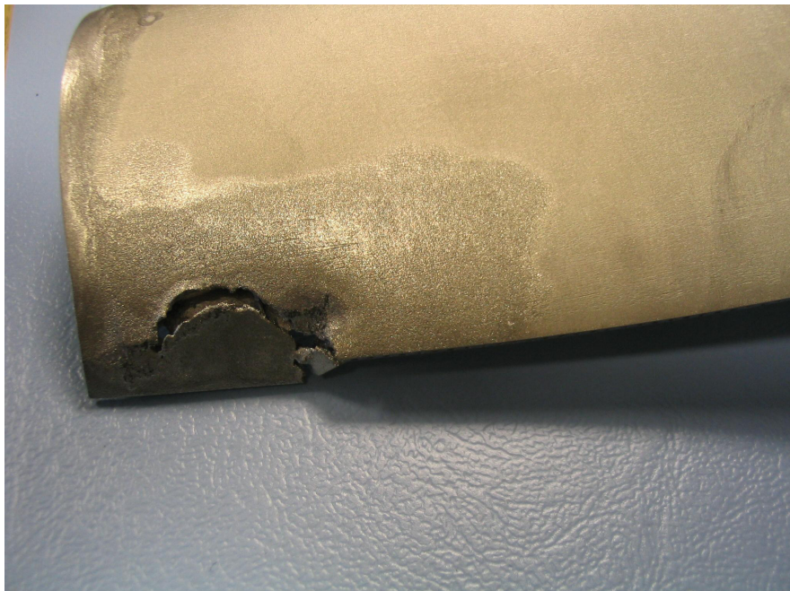
Fig. 5: The damaged IN738 blade
