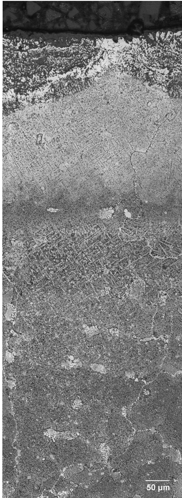
Fig. 1: LOM image showing the change in microstructure from surface to bulk. The specimen was etched using Kallings reagent.
