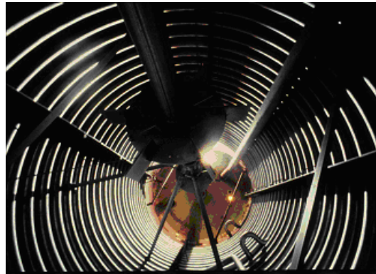
Figure 1.2. The inside of a stirred tank bioreactor. The impeller shaft with two 6-bladed Rushton turbines, baffles and internal cooling coils are seen in the picture. The picture was adopted from Nielsen et al. (2003)
