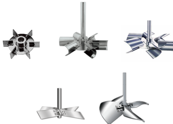
Figure 1.3. Selected impeller types. In the top row three different radial flow disc turbines are shown: A 6-bladed Rushton turbine (left), a Chemineer CD6 (middle) and a Chemineer BT6 (right), which is very similar in shape to the Scaba 6RSGT. In the bottom row a pitch blade turbine (left) and a Chemineer Maxflo W impeller (a high-solidity hydrofoil impeller) are shown.
