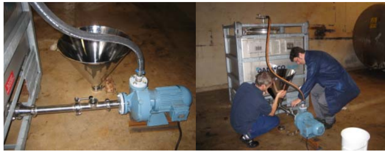
Figure A.3. Pallet tank used for dissolution of salt in syrup in the second experiment. The funnel is installed on the suction side of the pump and used to draw salt into the circulating syrup.
