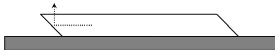
Figure 8.13: Light travelling down a waveguide terminated with a negative slope is coupled out vertically due to total internal reflection on the sloping sidewall.
