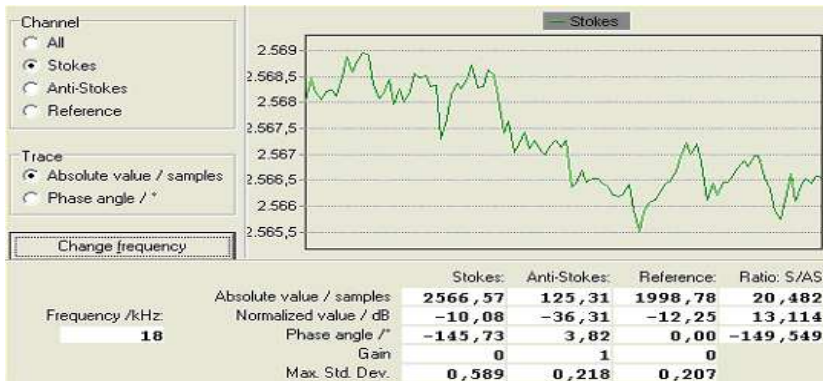
Figure F.3: Samples of square-modulated signal with 50% duty cycle over a period of time. Maximum standard deviation of the Stokes channel is 0.589.
