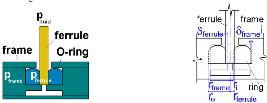
Figure 5-12: Schematic cross-sectional view of the plug'n'pump fluidic interconnection(left) and description of the parameters involved into the model (right)
