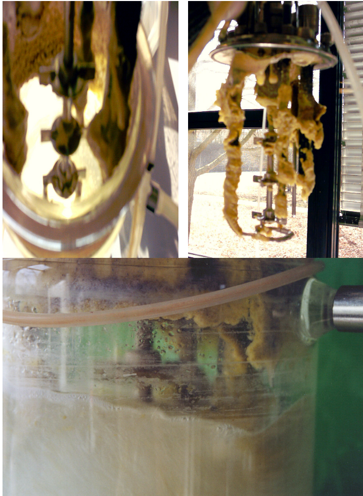
Figure 4.2 Unwanted growth and sporulation in fermenters during continuous fermentation.
