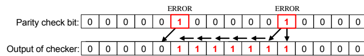
Figure 4.17: The output from the parity checker in case an error occurs in the header parity bit.
