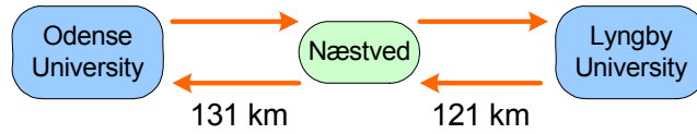
Figure 7.3: Distances between Odense and Lyngby. Both signals were optically amplified in Næstved.
