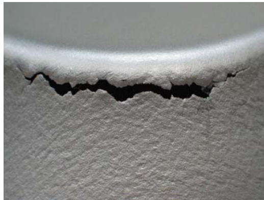
Figure 5: Fracture when forming the hyperboloid
