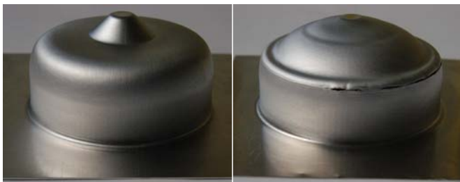
Fig. 6 Geometry after 4 stages of forming (left DDDU and right DUDD).
