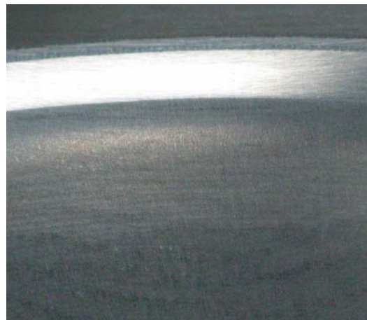
Figure 18: Surface quality in SPIF of 1.5 mm AA1050 H111 using a 0.63 mm DC04 steel dummy sheet
