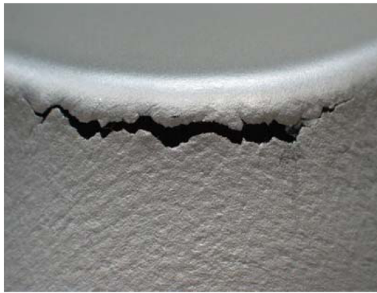
Fig. 35 Close up picture revealing no necking [42]
