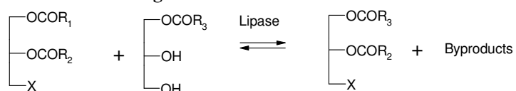
Figure 4.1: Reactions catalyzed by lipase for phospholipid modification
