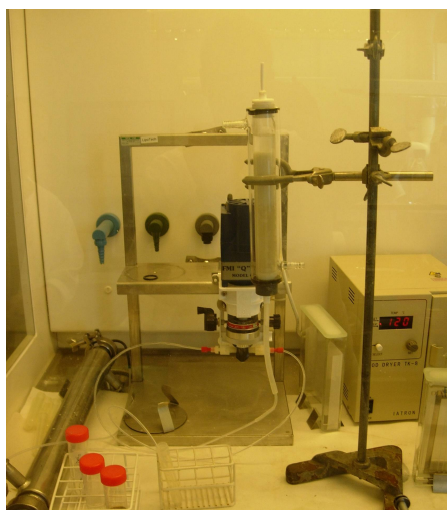
Figure 5.4: Set up for the column chromatography of structured phospholipids
