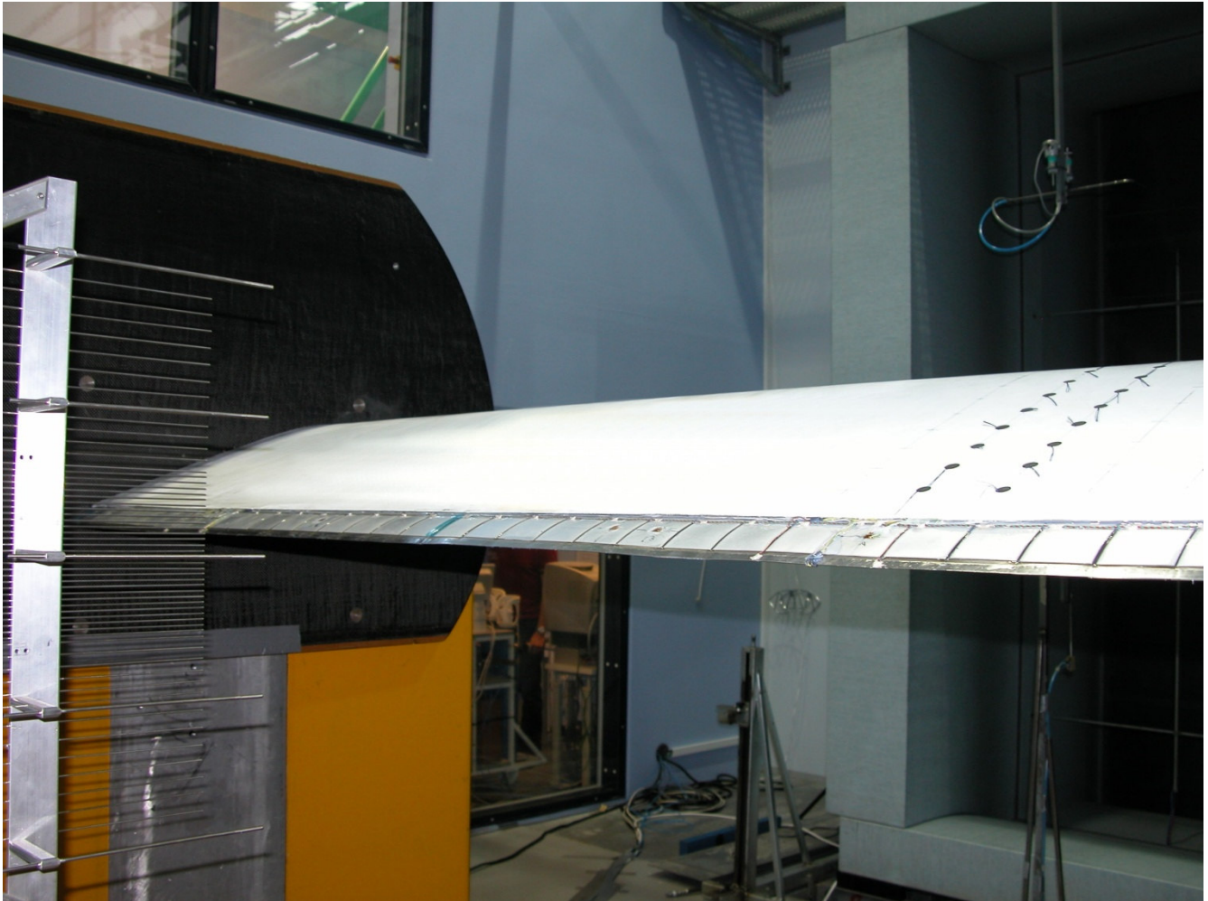
FIGURE C.2 THE TEST SECTION WITH THE TEST STAND AND THE WAKE RAKE DOWNSTREAM OF THE AIRFOIL SECTION.
