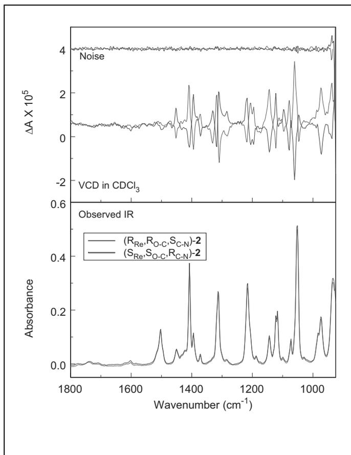
**Figure 4.** Observed IR (lower frame) and VCD (upper frame) of the two enantiomers of **2** in  $\text{CDCl}_3$ , 10 mg sample in 300  $\mu\text{L}$  solvent (58 mM);  $4 \text{ cm}^{-1}$  resolution; instrument optimized at 1400  $\text{cm}^{-1}$ ; collection time 12 h. IR spectra are solvent subtracted.
