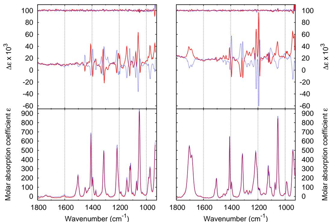
Figure 4.3: Observed IR (lower traces) and VCD spectra (upper traces, with the VCD noise level shown above) of each enantiomer of TpReO(ephedrine) (left) and TpReO(proline) (right) in  $CDCl_3$  solutions. Solvent IR spectra have been subtracted. The resolution was  $4\text{ cm}^{-1}$ , with the instrument optimized at  $1400\text{ cm}^{-1}$ . Collection time is 12 h. The region below  $925\text{ cm}^{-1}$  has been left out because of high solvent absorbance and thus higher noise.
