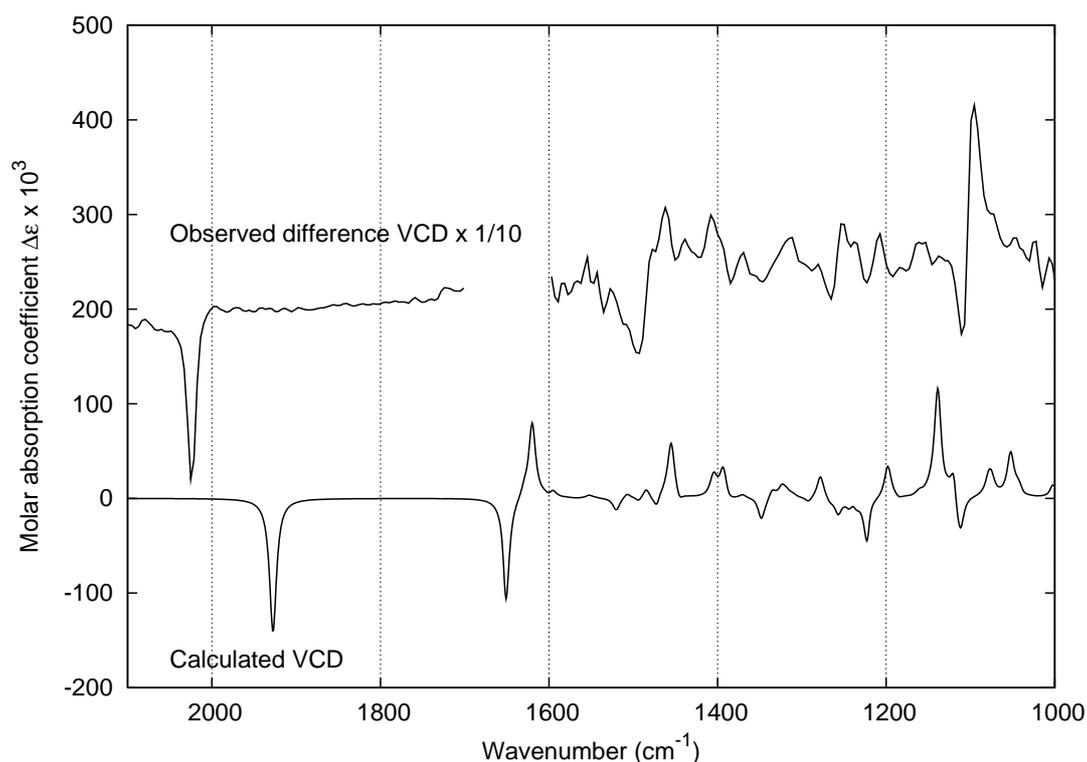
Figure 4.24: Experimental VCD difference of metMb-N<sub>3</sub> and metMb vs. calculated VCD of low-spin hemin-Im-N<sub>3</sub> at the DFT/B3LYP/LanL2DZ level, with frequency scaling factor 0.97 and HWHM=5 cm<sup>-1</sup>. The experimental resolution was 8 cm<sup>-1</sup>, and the acquisition time was 12 h for both samples, with the PEMs set at 1400 cm<sup>-1</sup>. The very noisy amide I region has been left out.
