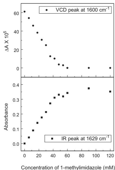
Fig. 21. Observed VCD intensity at 1600 cm<sup>-1</sup> (upper frame) and IR intensity at 1629 cm<sup>-1</sup> (lower frame) of (*R,R*)-CoSA in CDCl<sub>3</sub>(30mM) equilibrated with various concentrations of 1-methylimidazole in the presence of O<sub>2</sub>.
