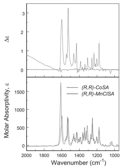
Fig. 3. Observed VCD (upper frames) and IR (lower frames) spectra of *(R,R)*-CoSA (5.4mg/154 $\mu$ L, 58 mM in CDCl<sub>3</sub>) and *(R,R)*-MnClISA (5.4mg/150 $\mu$ L, 57 mM in CDCl<sub>3</sub>); 92  $\mu$ m pathlength BaF<sub>2</sub> cell, instrument optimized at 1400 cm<sup>-1</sup>, 4 cm<sup>-1</sup> resolution and 1 h collection, scanning. Baselines corrected by subtraction of solvent spectra.
