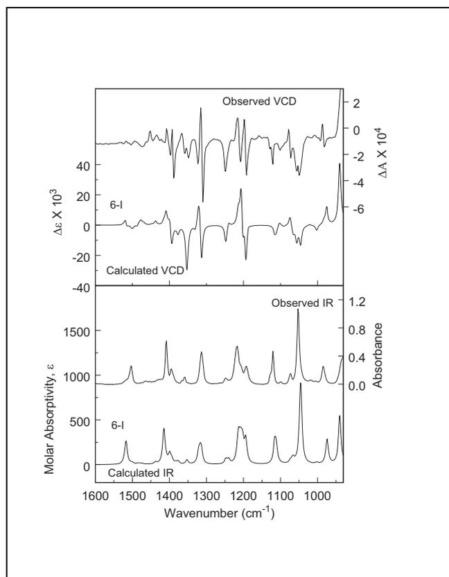
**Figure 16.** IR (bottom) and VCD (top) spectra for  $R_{\text{Re}}\text{-6}$ . Calculated spectra of the predominant conformer **6-I** (left axis; B3LYP/6-31G\*/Stuttgart; frequencies scaled by 0.97; bandwidth  $4\text{ cm}^{-1}$ ) compared to observed spectra for  $(-)\text{-6}$  (right axis;  $4.8\text{ mg}/100\text{ }\mu\text{L CDCl}_3$ ; solvent subtracted; resolution  $4\text{ cm}^{-1}$ ; instrument optimized at  $1400\text{ cm}^{-1}$ ; collection time is 12 h).
