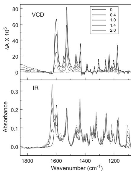
Fig. 19. Observed VCD (upper frame) and IR (lower frame) spectra of (*R,R*)-CoSA (30 mM) equilibrated with 0 to 2 molar equivalents of 1-methylimidazole as indicated, in the presence of  $\text{O}_2$ ; 0.10 mm pathlength  $\text{BaF}_2$  cell, 1 hour collection, 4  $\text{cm}^{-1}$  resolution, PEM optimized at 1400  $\text{cm}^{-1}$ . Spectral baselines corrected by subtracting solvent spectra.
