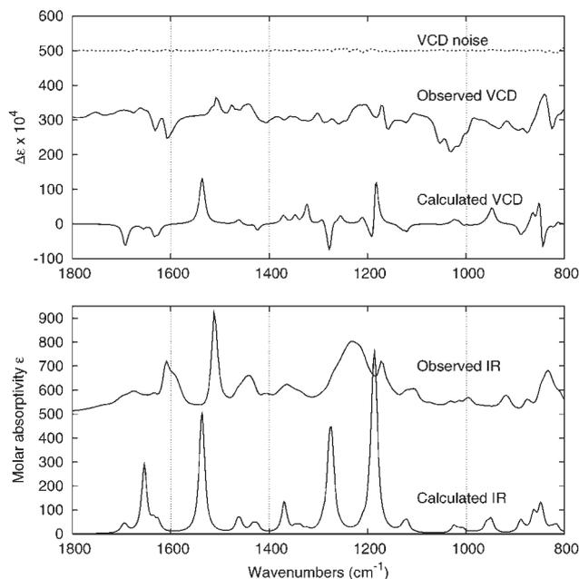
**Figure 5.** Observed IR absorption (lower half) and VCD (upper half) spectra of nyasol in a KBr pellet, compared to the DFT calculation for (*S*)-nyasol using B3LYP/AUG-cc-pVDZ. The experimental resolution is 8 cm<sup>-1</sup>, with the instrument optimized at 1400 cm<sup>-1</sup>. The total acquisition time is 31 h, and spectra from two different orientations of the KBr pellet were averaged to reduce the baseline offset. VCD noise is shown in the uppermost (dashed) trace.
