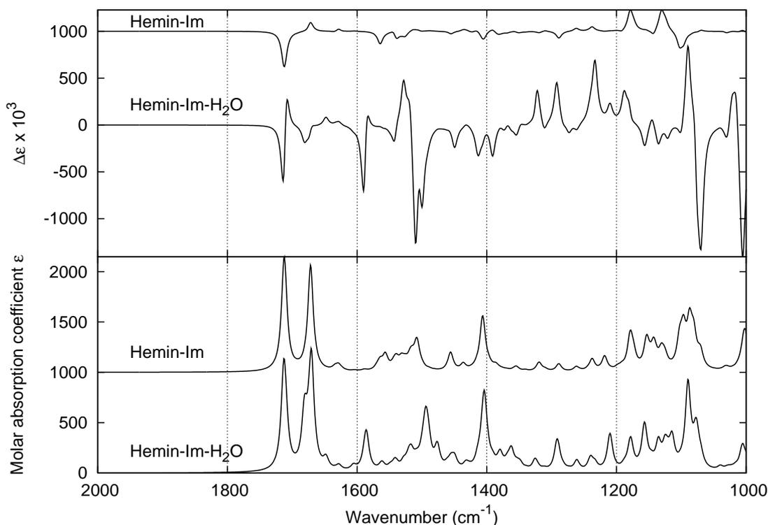
Figure 4.29: Calculated IR (bottom) and VCD (top) of HS Fe(III) hemin with proximal Im and either distal H<sub>2</sub>O or no distal ligand, calculated using B3LYP/LanL2DZ.
