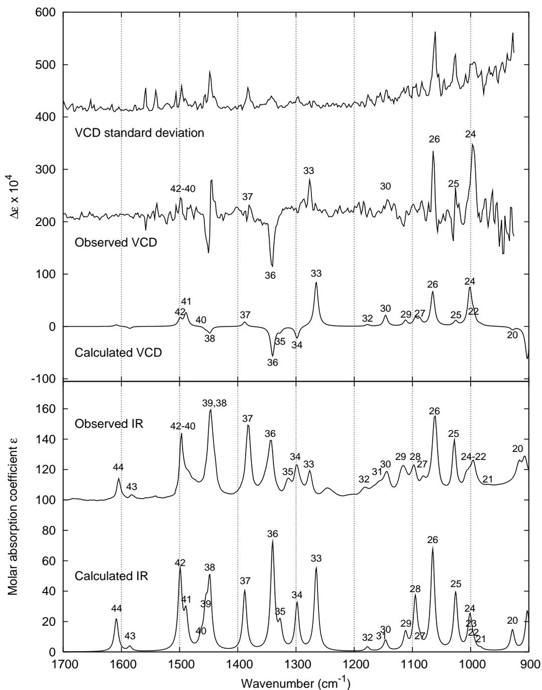
Figure 3.3: Comparison of experimental and calculated IR (bottom) and VCD (top) spectra of  $\alpha$ -methylphenyloxirane. Calculated spectra are for the (*R*)-enantiomer with 95% *ee*, using B3LYP/aug-cc-pVTZ with an implicit solvent model, using 4  $\text{cm}^{-1}$  half-width and a frequency scaling factor of 0.98. Most fundamentals are numbered. Experimental spectra are of neat samples, measured for 8 h using 4  $\text{cm}^{-1}$  resolution and a 17.3  $\mu\text{m}$  path length.
