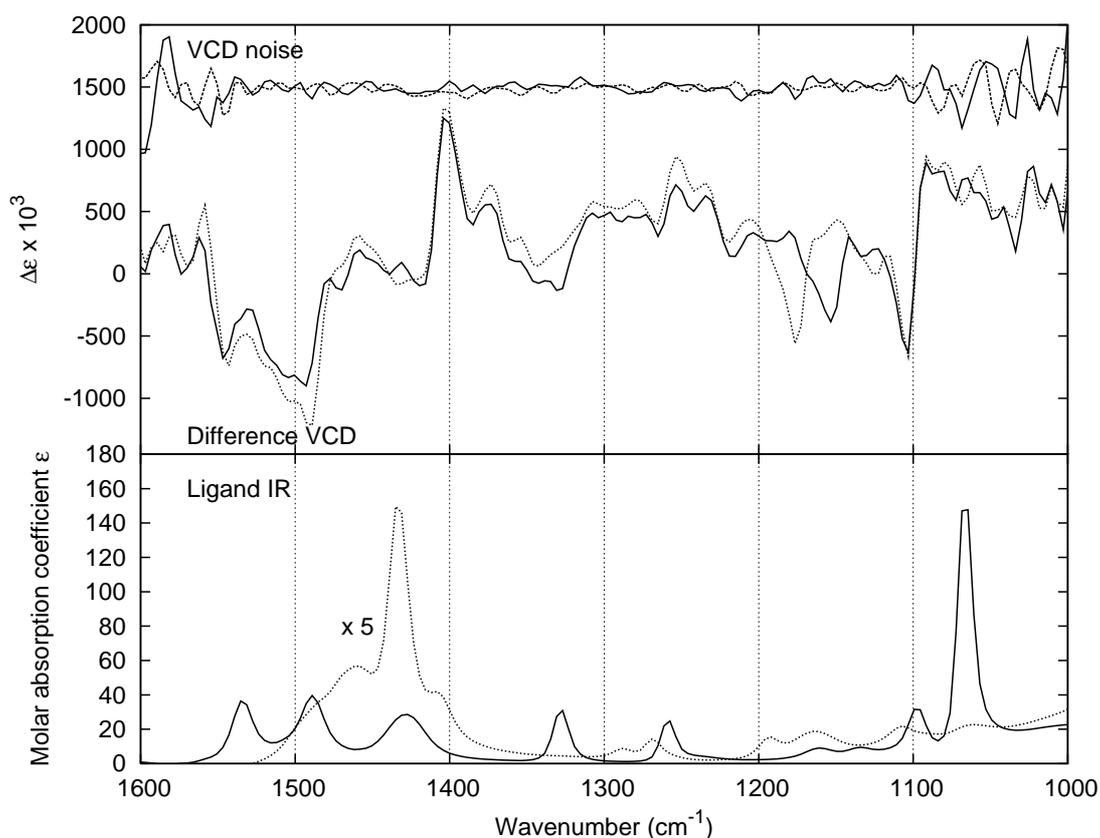
Figure 4.20: Experimental VCD difference (metMb subtracted) spectra of metMb-Im (—) and metMb-Im- $d_3$  (····) (top), compared to IR spectra of ligands Im (—) and Im- $d_3$  (····) (bottom) in 0.44 M and 1.8 M solutions, respectively. The resolution is  $8\text{ cm}^{-1}$ , with the PEMs set at  $1400\text{ cm}^{-1}$ . All spectra are solvent subtracted. An optical filter with cutoff above  $2000\text{ cm}^{-1}$  was used.
