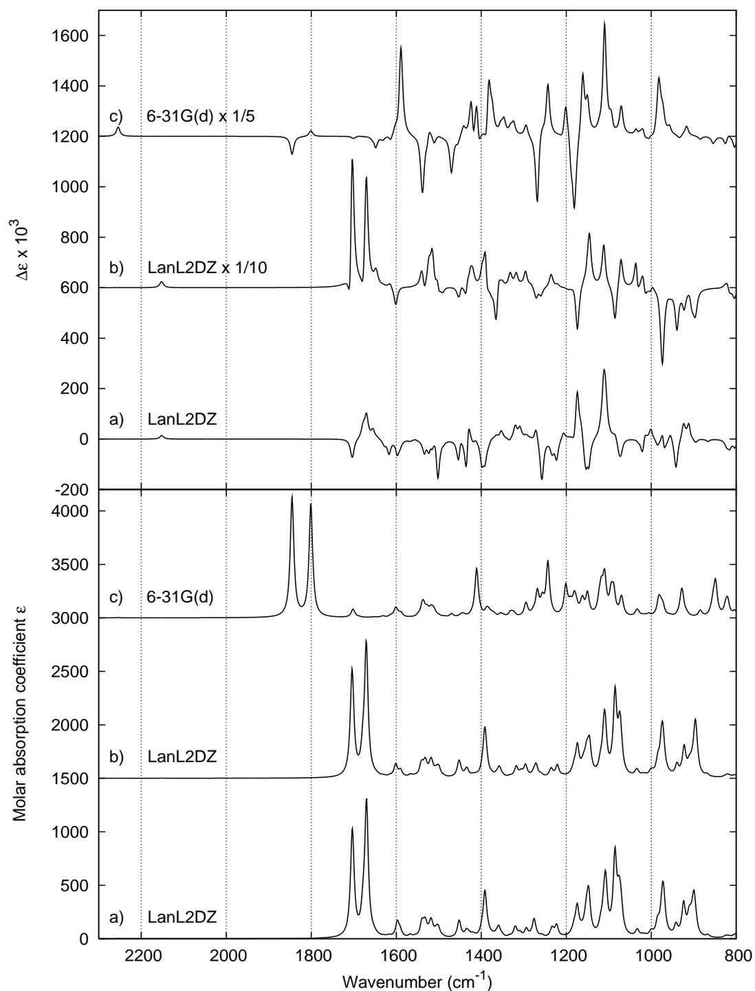
Figure 4.26: Calculated IR (lower half) and VCD (upper half) spectra of low-spin hemin with proximal Im and distal cyanide. The DFT/B3LYP level was used with basis sets as indicated and Lorentzian broadening ( $\text{HWHM}=5\text{ cm}^{-1}$ ) without frequency scaling. a) With Im rotated  $90^\circ$  off from 1EBC His93. b) With Im oriented as 1EBC His93. c) With Im rotated  $45^\circ$  off and 1 imaginary frequency (Fe-C $\equiv$ N bending mode).
