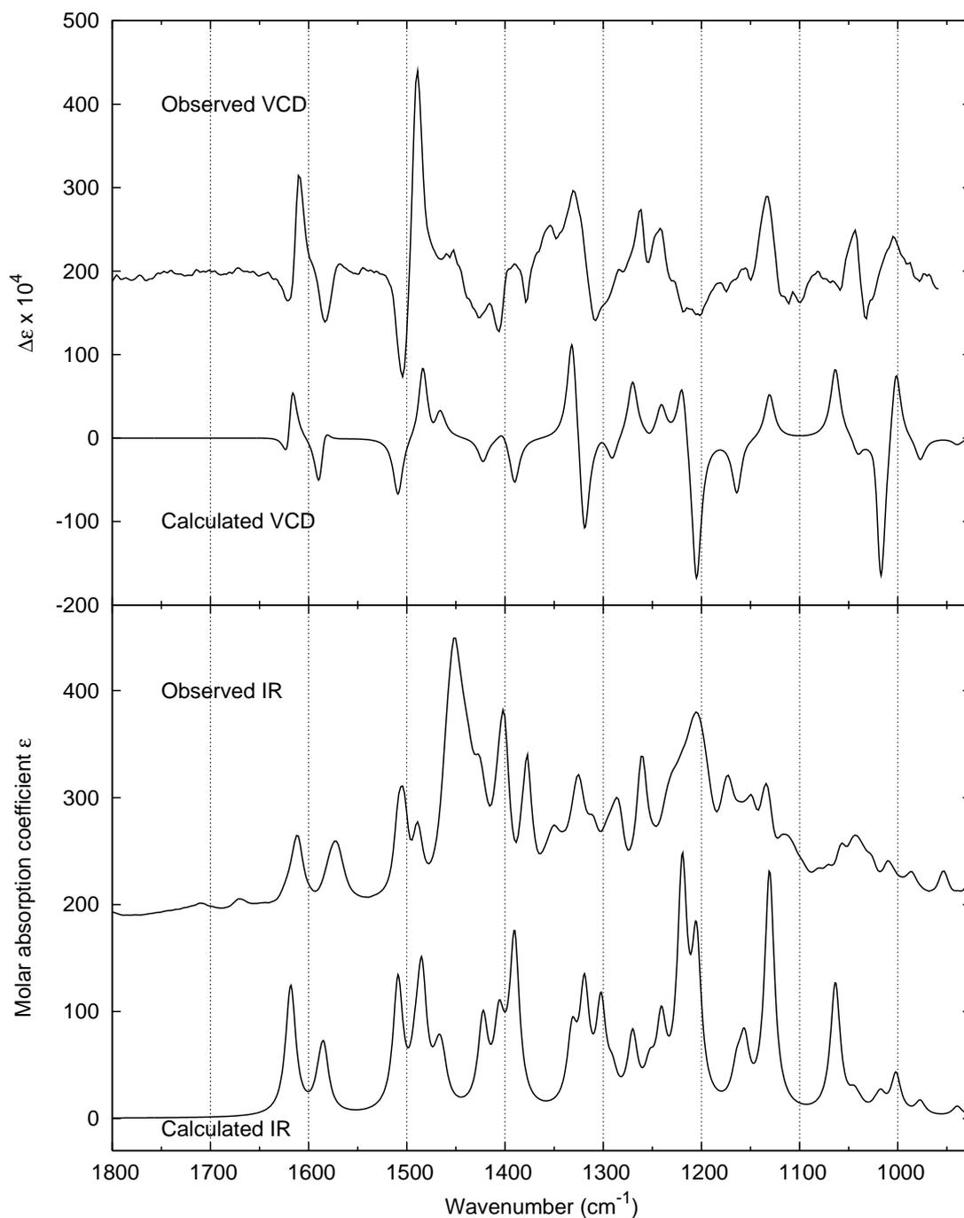
Figure 3.16: Observed IR spectrum (bottom) and difference VCD ( $\#2 - \#1$ )/2 of the atropisomers (top) vs. DFT calculated spectra for the (*P*)-atropisomer of the model compound in Figure 3.13, using B3LYP/6-31G(d). Experimental conditions are given in Table 3.1.
