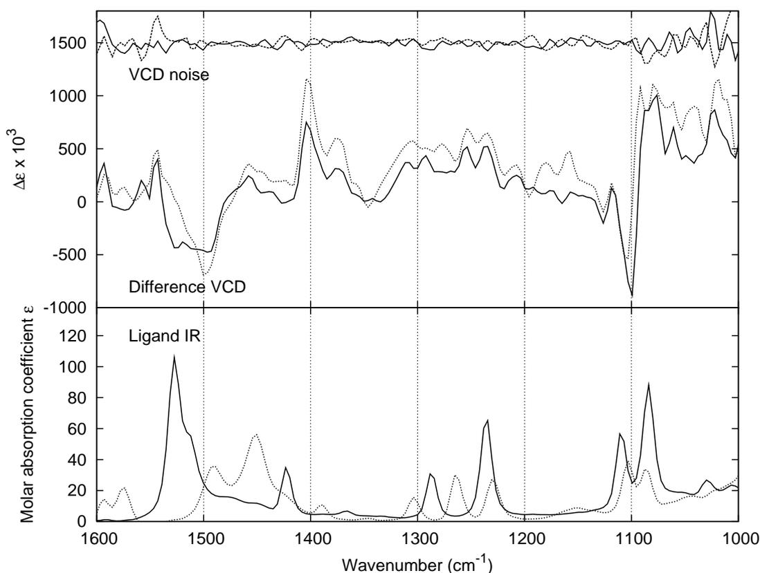
Figure 4.21: Experimental VCD difference (metMb subtracted) spectra of metMb-1-Me-Im (—) and metMb-4-Me-Im (····) (top), compared to IR spectra of ligands 1-Me-Im (—) and 4-Me-Im (····) (bottom) in 1.9 M solutions. The resolution is  $8\text{ cm}^{-1}$ , with the PEMs set at  $1400\text{ cm}^{-1}$ . All spectra are solvent subtracted.
