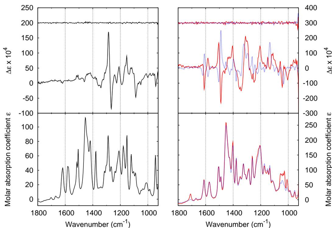
Figure 3.15: Observed IR (lower traces) and VCD spectra (upper traces, with the VCD noise level shown above) of (*S*)-curcuphenol (left) and its dimers (right), #1 (—) and #2 (····). Experimental conditions are given in Table 3.1 above. Solvent spectra are subtracted, and absorbance converted into molar absorption coefficient using Lambert-Beer's law (2.30).
