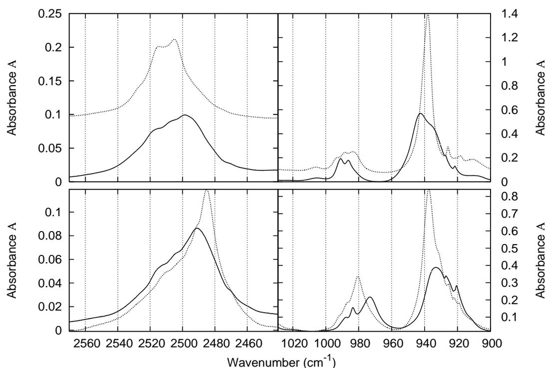
Figure 4.8: Experimental IR spectra of Re(V) complexes (*R,R,S*)-1 (bottom) and (*R,R*)-2 (top) in  $\text{CHCl}_3$  (—) and KBr pellets (···), showing the B–H stretching (left) and Re=O stretching regions (right). The resolution is  $0.25 \text{ cm}^{-1}$ , and the collection times 90 min.
