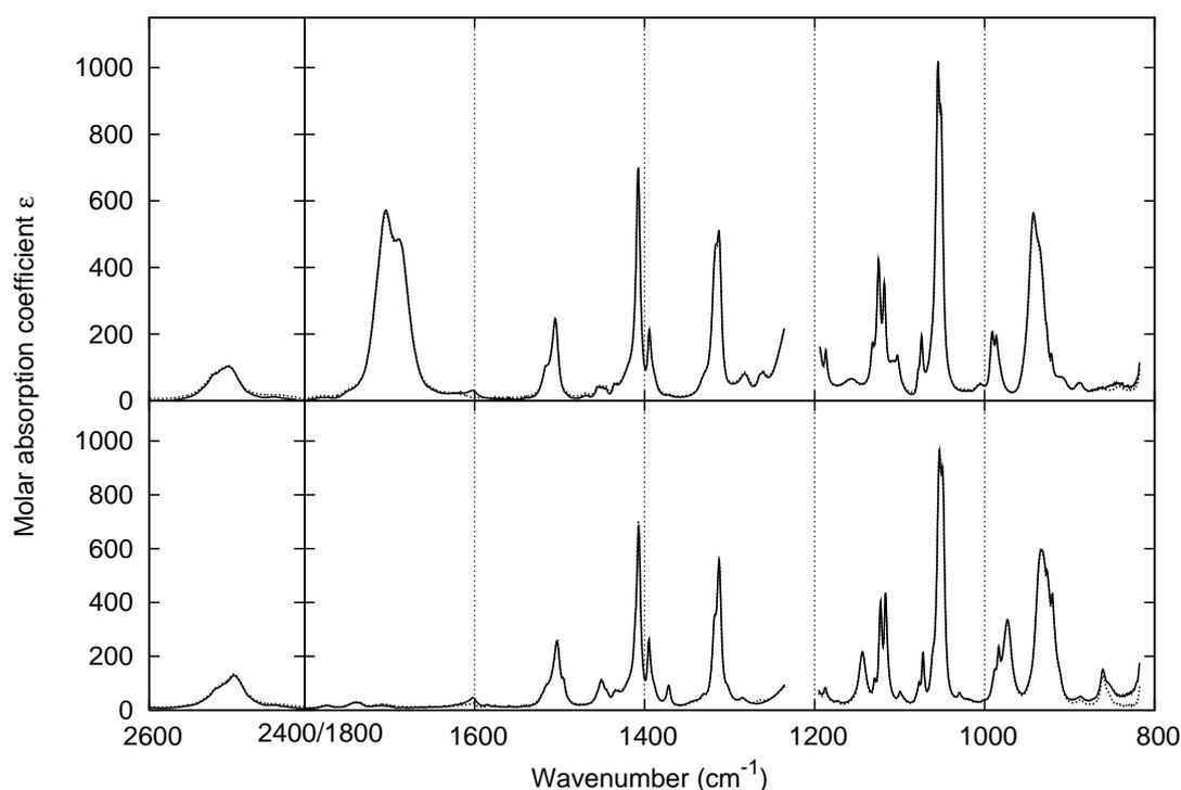
Figure 4.9: Experimental IR spectra of Re(V) complexes (*S,S,R*)-**1** (bottom) and (*S,S*)-**2** (top) in  $\text{CHCl}_3$ , using lower (—) and normal (⋯) concentrations (1: 61 mM vs. 4.3 mM; 2: 95 mM vs. 4.7 mM). The intense  $\text{CHCl}_3$  band around  $1200\text{ cm}^{-1}$  has been blanked. The resolution is  $1\text{ cm}^{-1}$ , and the collection times 35–90 min.
