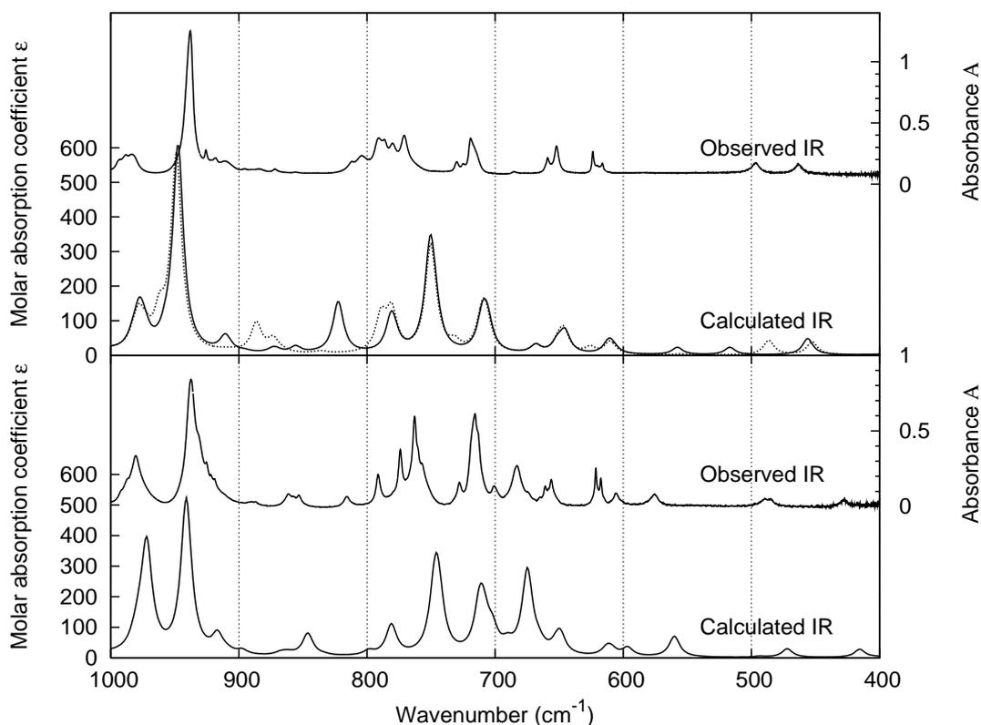
Figure 4.7: Experimental vs. calculated IR spectra of Re(V) complexes (*R,R,S*)-1 (bottom) and (*R,R*)-2 (top) in KBr pellets, showing the 400–1000  $\text{cm}^{-1}$  region compared to the B3LYP/6-31G(d)/Stuttgart RSC 1997 ECP calculations. Both conformers **2a** (—) and **2b** (····) are included. The experimental resolution is 0.25  $\text{cm}^{-1}$ , and the collection times 90 min.
