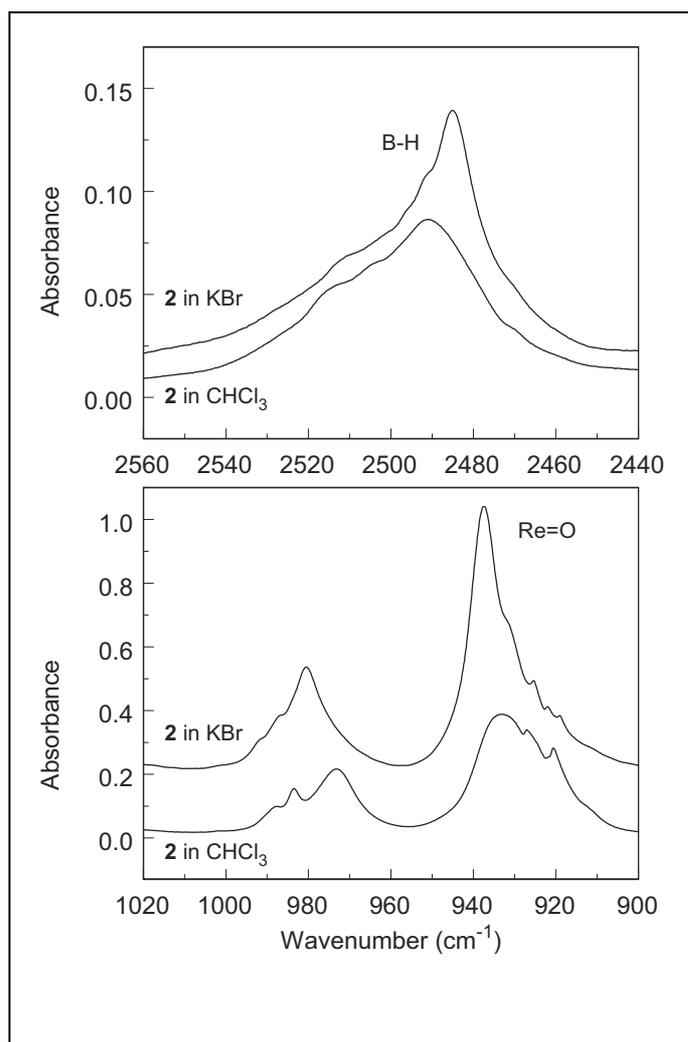
**Figure 6.** Higher resolution IR spectra of **2** in CHCl<sub>3</sub> solution and in a KBr pellet, showing the B-H stretching (top) and Re=O stretching regions (bottom). Resolution 0.25 cm<sup>-1</sup>; collection time 90 min. KBr spectra are offset for clarity.
