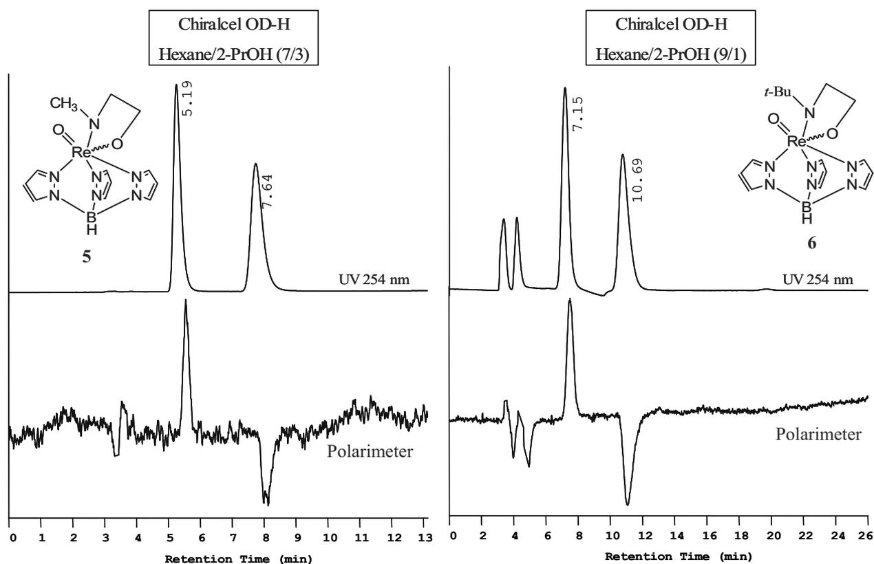
**Figure 2.** Analytical chiral HPLC chromatograms for the separations of compounds **5** and **6** on Chiralcel OD-H, with hexane/2-PrOH (7/3) as mobile phase at 1 ml/min for **5**, and hexane/2-PrOH (9/1) for **6**, and with UV (254 nm) and polarimetric detectors.
