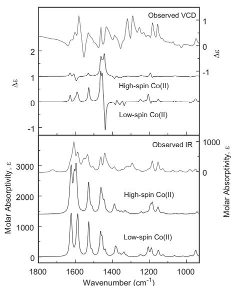
Fig. 18. Comparison of VCD (upper frame) and IR (lower frame) spectra observed for (*R*)-CoSalbinapht (right axes) with calculated spectra for the high- and low-spin Co(II) complexes (left axes). Observed spectra were obtained under conditions in Figure 16. Calculations of the VCD and IR spectra carried out with Gaussian 03 at DFT level with B3LYP functional and 6-31G(d) basis set for C, N, O, H and Ahlrich VTZ basis set for Co(II).
