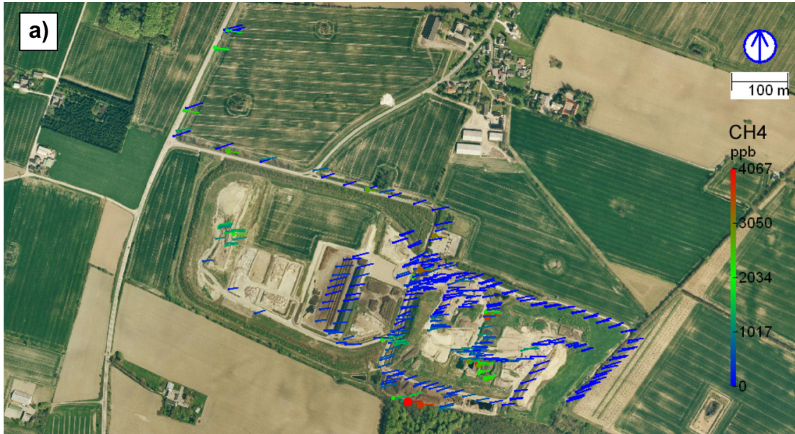
Fig. 4.4 CH 4 leak survey with FTIR across the Fakse landfill and composting area on of October 11, 2006. Color scale and dot size indicate concentration of CH 4 in ppb, sampled 2 m above ground. The scale is linear
