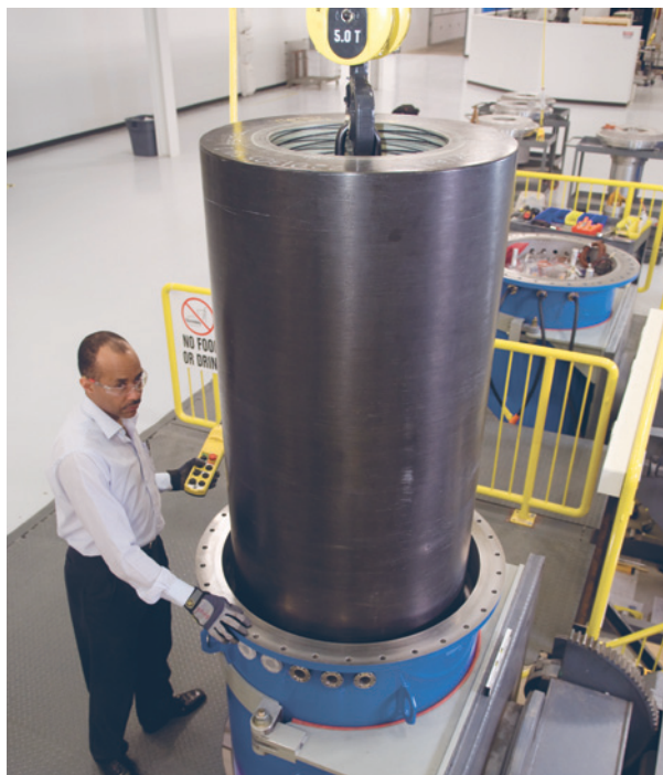
Figure 34: 100 kW/25 kWh Beacon flywheel unit. The flywheel is sealed in a vacuum chamber and spins at 8,000-16,000 rpm (source: Beacon Power, www.beaconpower.com )
