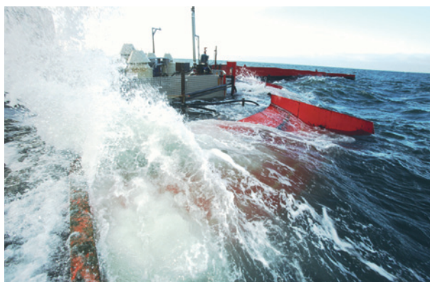
Figure 25: Wave Dragon 01:04.5 prototype during testing in Nissum Bredning (© Earth-vision.biz)
