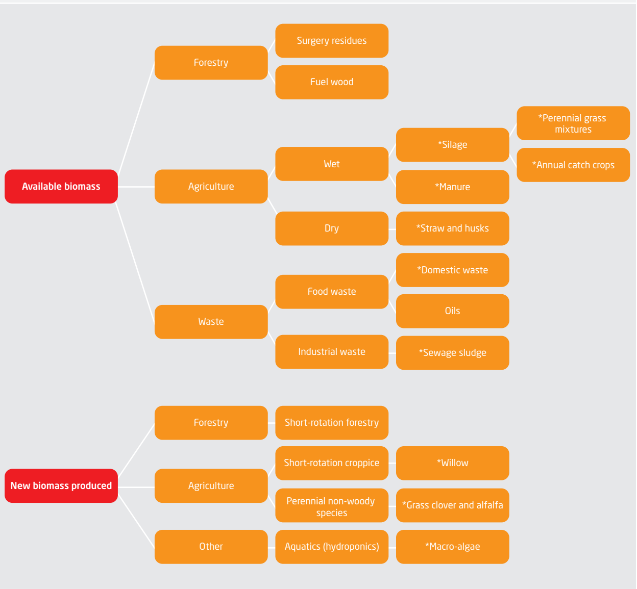
Figure 28 Sources of already available (top) and potential new (above) biomass for sustainable bioenergy
