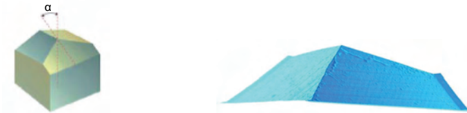
Figure 6.4: The Berkovich pyramid as schematic (left) and measured (right).
