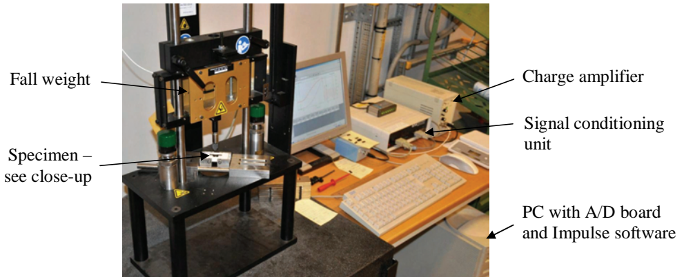
Figure 11.2: Falling weight impact tester at NNAS. Close-up shown in Figure 11.3.
