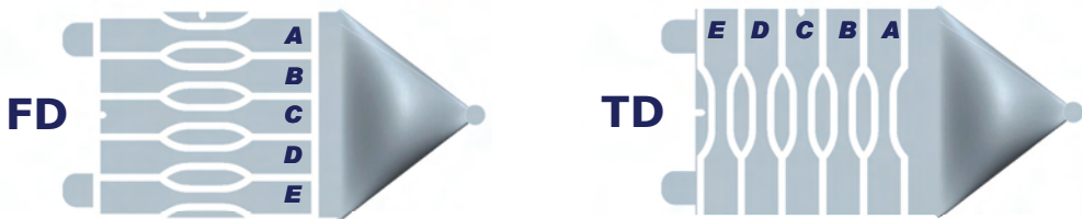
Figure 7.6: Dumbbell-shaped specimens for tensile testing.
