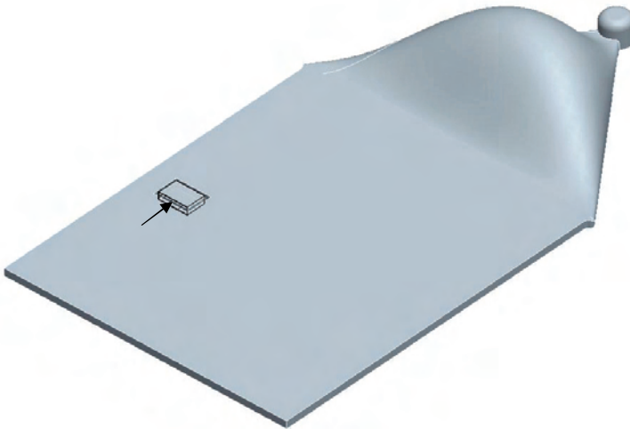
Figure 6.9: Position of indentation sample and tested cross-section in the moulded test blank.
