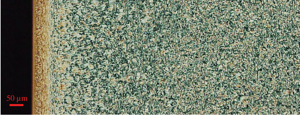
Figure 7.4: PLM micrograph from the original 10 μm thin section of the plate from process condition VF&W (chapter 4.1), taken at same magnification as used in Figure 7.5 (100X).
