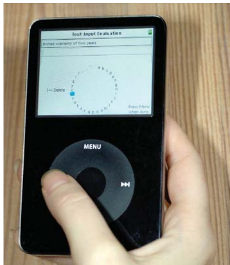
Figure 4.5: The TUP iPod prototype and the Text Entry Evaluation Tool.
