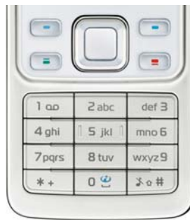
Figure 2.2: Keyboard from Nokia 6300. Besides the 12 keys ITU-T keyboard there is also keys for navigating the user interface and call handling.
