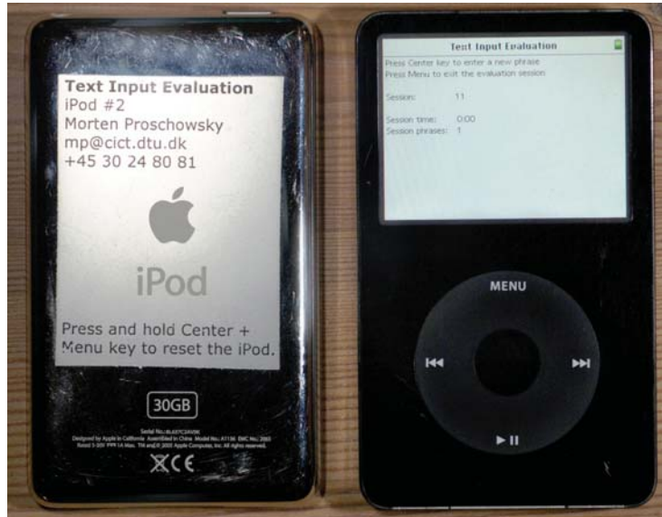
Figure 4.6: The TUP iPod prototype. The left image shows the back of the iPod. The right image shows the main screen in the Text Entry Evaluation Tool.
