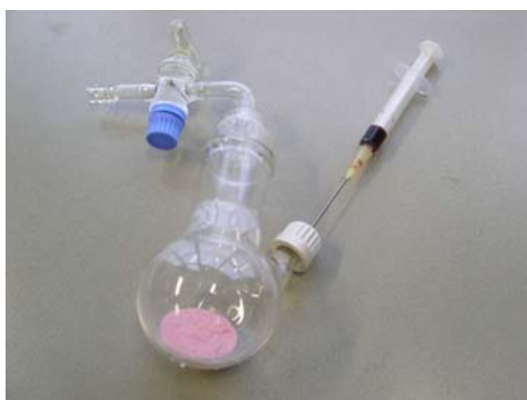
Figure 10.1 Catalyst preparation, incipient wetness impregnation of silica with a cobalt-manganese containing solution under vacuum.
