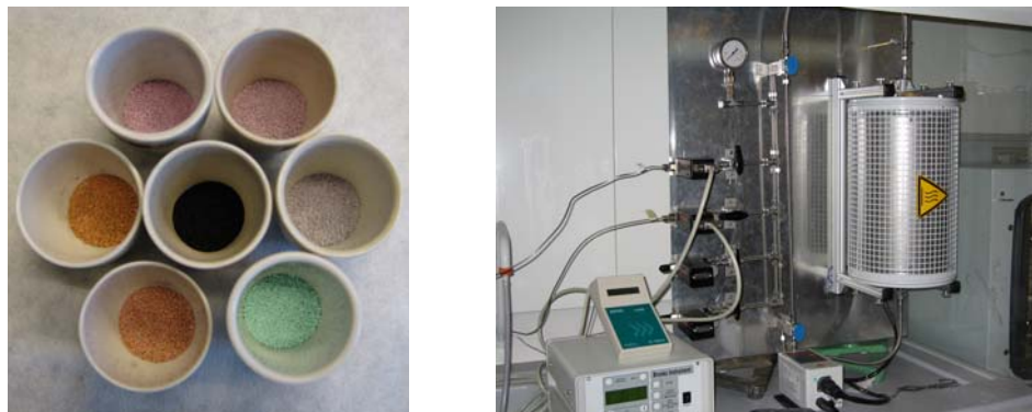
Figure 4.1 Nickel, iron, cobalt, and bimetallic catalysts before calcination are shown standing around one calcined sample (left). One of the three activity test set-up used for the methanation experiments in this study (right).
