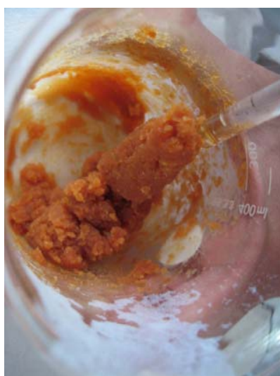
Figure 12.2 The red gel obtained by introducing iron directly during the synthesis of the BEA zeolite, is considerable more viscous than the gel obtained during the synthesis of the conventional H-BEA zeolite.
