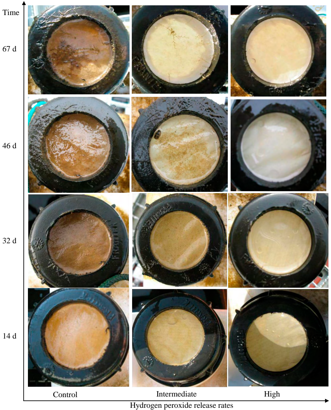
Figure 6.9: Pictures of the flux membranes after 14 (bottom series), 32 (middle), 46 days, and 67 days immersion in Jyllinge Harbour. From left to right: reference membrane (control), 224 \mu\text{g}/(\text{cm}^2\cdot\text{day}) and 2800 \mu\text{g}/(\text{cm}^2\cdot\text{day}) hydrogen peroxide release rates.
