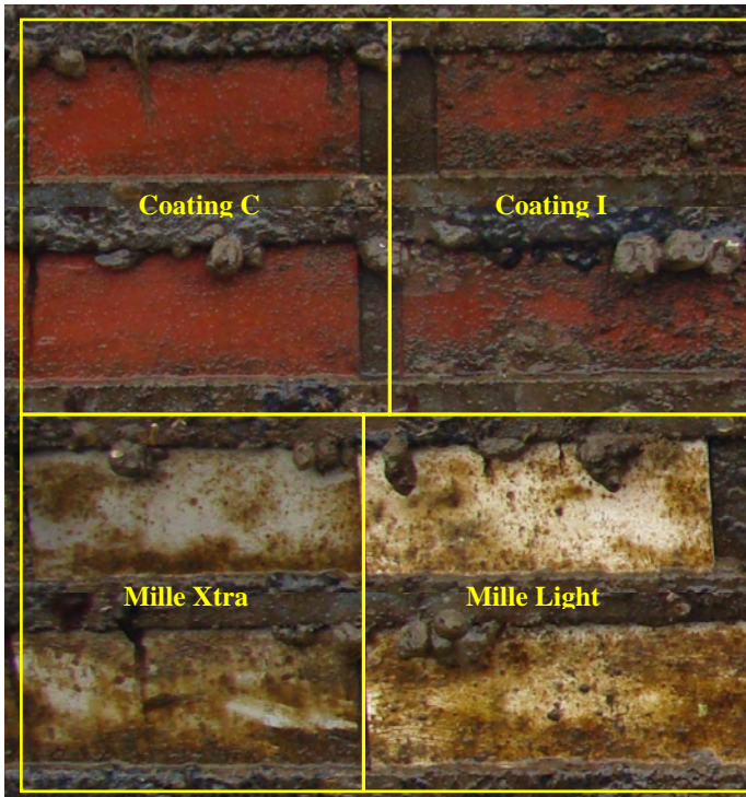
Figure 5.8: Photos of coated panels tested in the North Sea after 67 days immersion. Each coating is shown with a replicate, but they were not mounted on the raft with the same proximity. Photo modified from Kristensen et al. (2009b).
