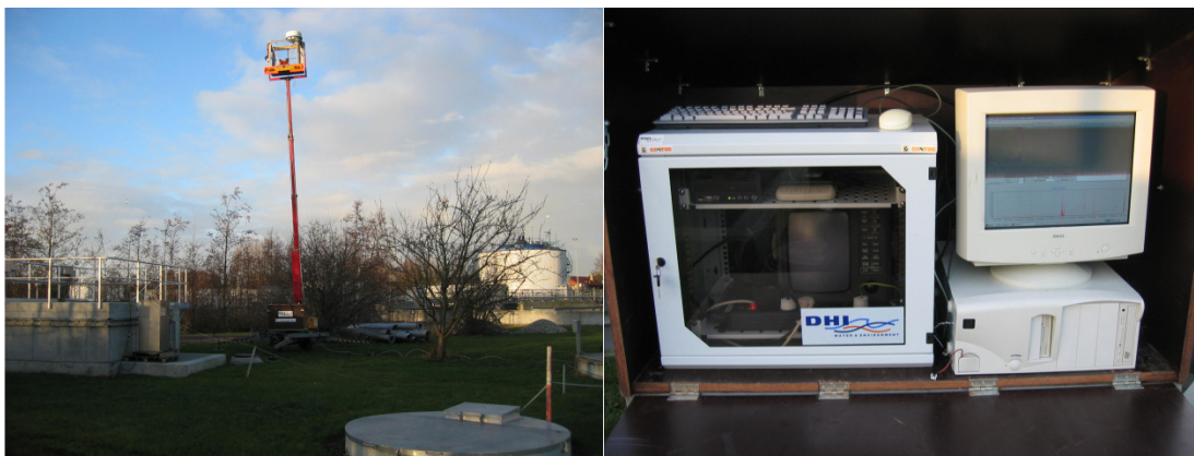
Figure 5.11 Example of site location test with use of a 2 kW X-band radar mounted on a mobile lift to the left. On the right a look at the mobile signal processing unit used for site locations.
