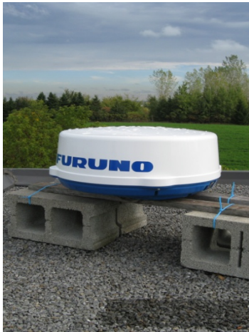
Figure 5.3 City-LAWR installation. Temporary installation at J. S. Marshall Radar Observatory, McGill University in the fall of 2007.
